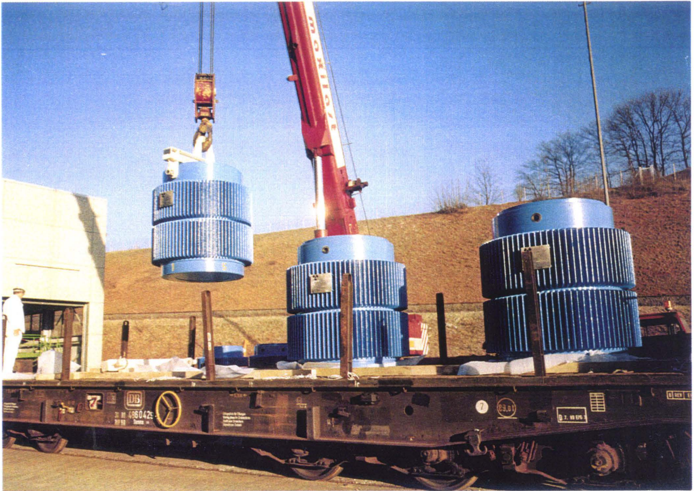
Fig. 13: Delivery of the Empty Multiple Transport Cask, Castor GSF-5
