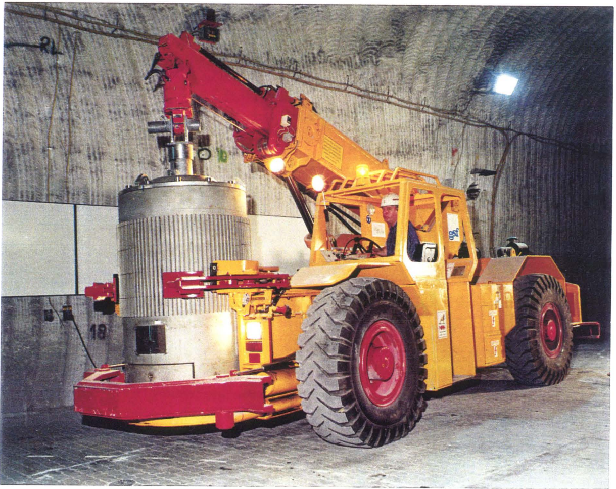
Fig. 30: Gallery Transport Vehicle, Sirius, with Single Transport Cask, Asse TB1
