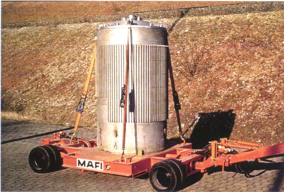
Fig. 11: Heavy-Duty Trailer with Lashed Single Transport Cask, Asse TB1
