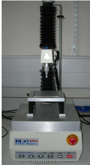
Figure 2.26 TA-XT2i, texture analyser from Stable Micro System, UK, used to obtain puncture force results for carrot pieces, following rehydration.
