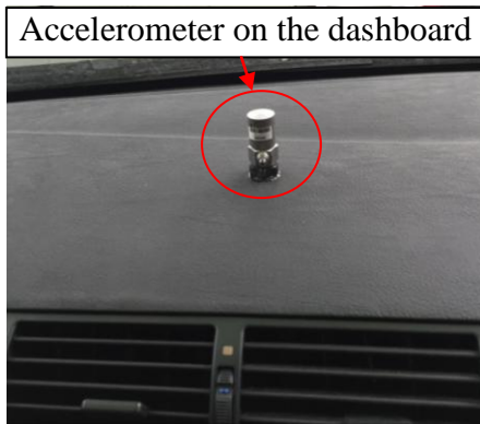
Figure 6-15: Measurement of the dashboard vibration in vehicle B
