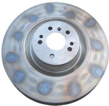
Figure 2-2: One brake disc with “hot spots” under cold status 56
