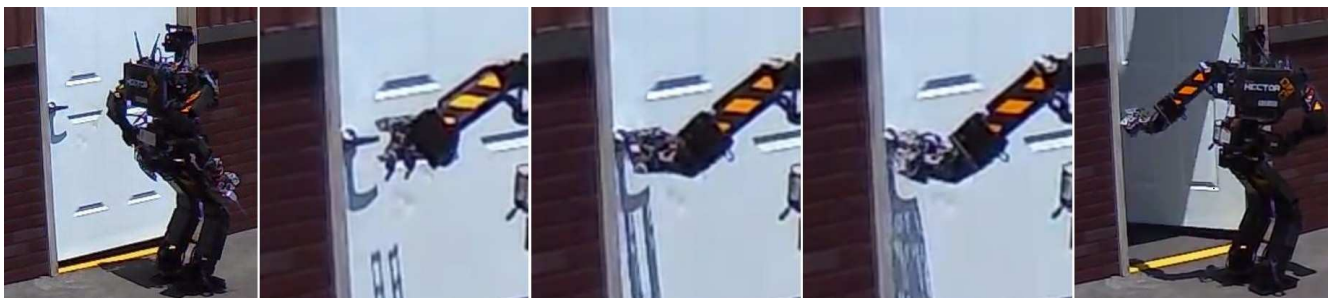
Figure 9.6: The THOR-MANG robot of Team Hector opening the door at DRC Finals Day 1. Images courtesy of Alberto Romay.
