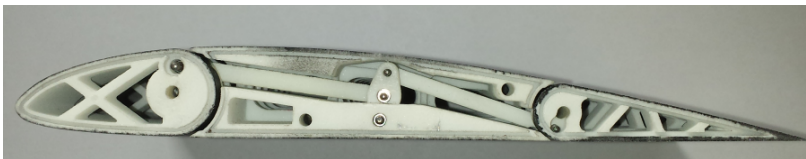
Figure 4.3.: Picture of the adaptive camber airfoil model used in the Oldenburg active grid wind tunnel experiments. The two rod coupling mechanism is chosen to minimize backlash and is restrained by a spring system (not shown).
