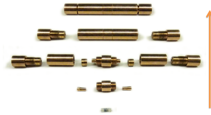
Figure 3.4: Sequence of the assembly of the pressure cell for magnetization measurements.
