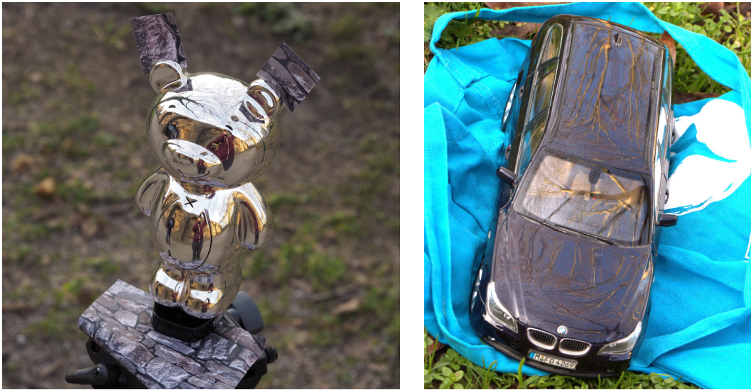
Figure 4.8: Left: A photograph of the TEDDY dataset which consists of a highly specular surface with only little structure. Paper strips were attached to the object to provide enough diffuse features for SfM. Right: The MODEL CAR dataset has more structure on it but consists of parts with lower surface curvature.
