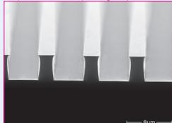
4 µm ma-P 1240, 3 µm Stege, 5 µm Gräben
