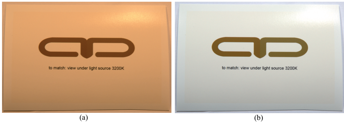
Figure 4.16.: A captured spectral print representing metamers and non-metamers under the 3200K and D65 illuminations respectively. The embedded light sources of the Caddon viewing booth were utilized. Please note that the printing and capturing process can lead to color errors. The results are more reliable in the zoomed-in electronic version of this dissertation.
