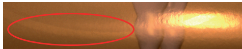
Figure 6.2.: A cutout of an image captured from a printout representing gloss-differential artifacts (visible banding in the marked ellipse) occurred due to variations in deposited ink area coverage.
