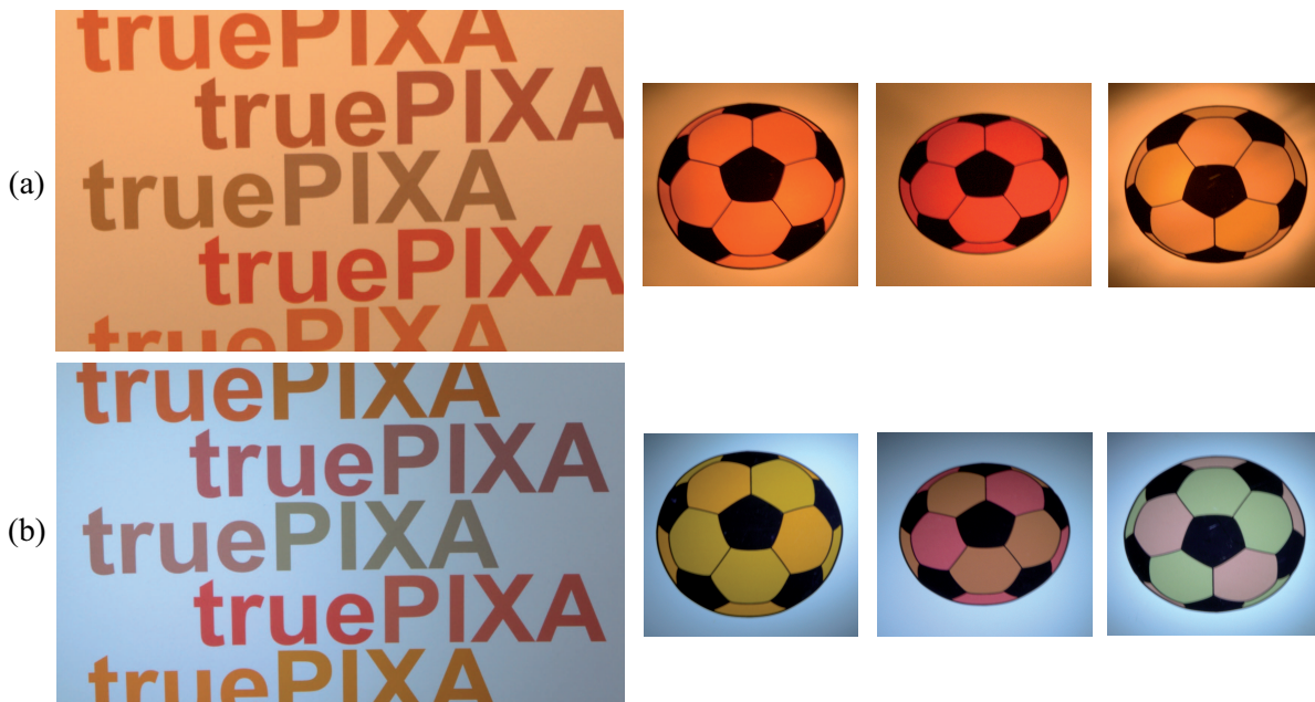
Figure 4.17.: Captured spectral prints under two light sources: (a) halogen-based and (b) LED-based flashlights. Noticeable color changes are visible in the samples of the second row. Please note that the printing and capturing process can introduce color errors. The results are more reliable in the zoomed-in electronic version of this dissertation.
