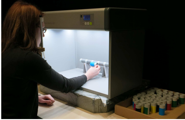
Figure 6.24.: Gloss scaling experimental setup. This figure has been taken from [SBU14].
