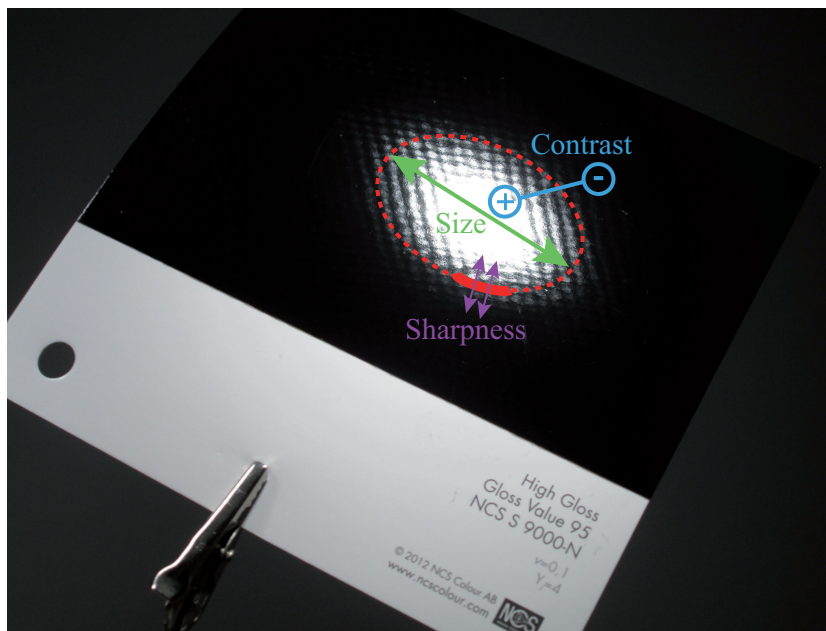
Figure 5.4.: Some of the proximal gloss cues related to specular highlights according to Marlow et al. [MKA12].
