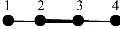
Figure 3.3: A linear chain of four qubits with nearest-neighbour interactions, where the inner coupling is twice as strong as the two outer couplings.
