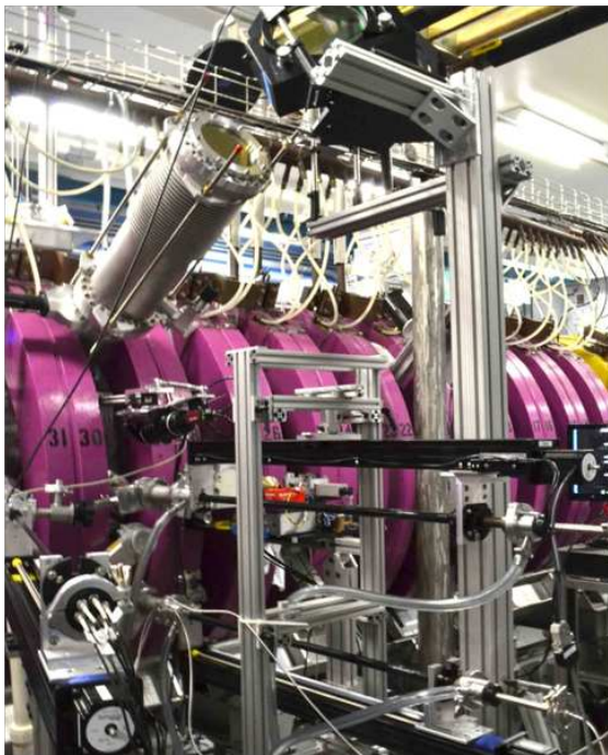
Figure 3.5: Left: The setup of the final focusing lens for Raptor laser beam injection into the LAPD. Right: Three-dimensional layout of the experiment performed inside of the LAPD. The laser beam irradiates the graphite or high-density polyethylene ( C_2H_2 ) target which is located 30 cm off the LAPD-coordinate center and creates a dense plasma that expands into the tenuous ambient plasma in the LAPD. Probes are placed either across (perpendicular probe) or along the field (parallel probes) and measure magnetic and electric field fluctuations. Extracted from [Niemann et al., 2013].
