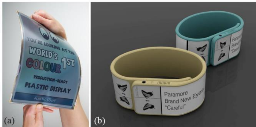
Figure 2.1: Two examples on application of flexible electronics in new products: (a) A flexible color display [72] that is already available, and (b) a wraparound display [71] as a concept design for wearable devices.
