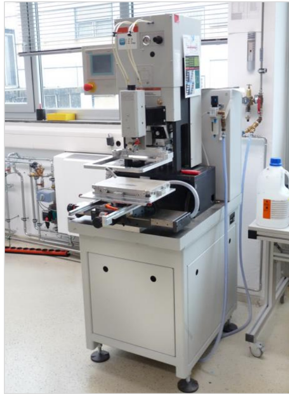
Figure 4.15: Screen printing machine Kammann-K15Q SL at IDD, that applied for printing the samples.
