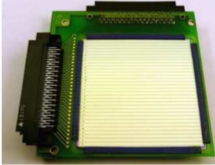
Figure 2.6: Photograph of the DSSSD target detector mounted on its PCB frame [5].
