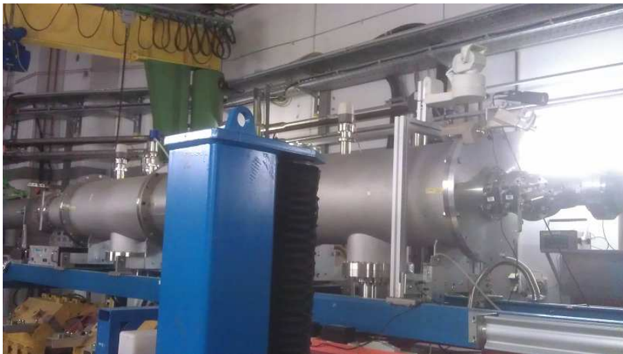
Figure C.1.: The removal of part of the beam line results in an larger time-of-flight distance and therefore better energy resolution.
