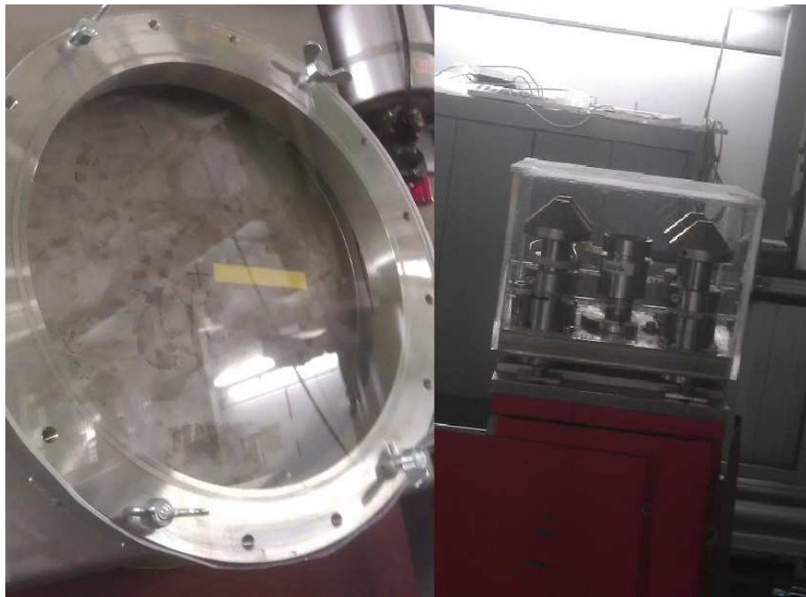
Figure B.1.: The closed beamdump (left) covered by a plastic cover and the optical stand (right), used for beamline alignment are reasonable candidates for backscattering as well as an additional source of fragmentation.
