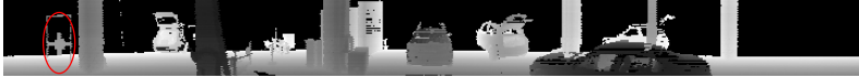
Figure 1: Example of rasterized depth map, as seen from the 3D LRF virtual center. In red: Target used for manual selection of keypoints.
