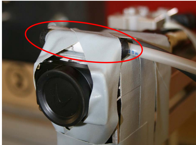
Fig 4.18: Dosimeter (red ellipse) mounted on the CCD camera.
