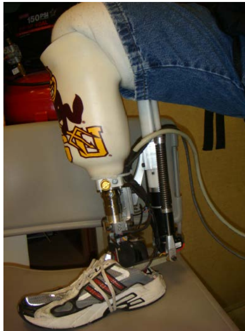
FIGURE 1.9: The SPARKy (Spring Ankle with Regenerative Kinetics) robot. This design uses a DC motor with a spring [28].
