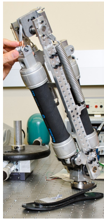
FIGURE 1.11: The Rocket powered prosthetic foot developed by Goldfarb from Vanderbilt University (US) [29].
