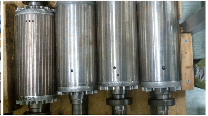
(b) Holes drilled to create artificial broken bars
