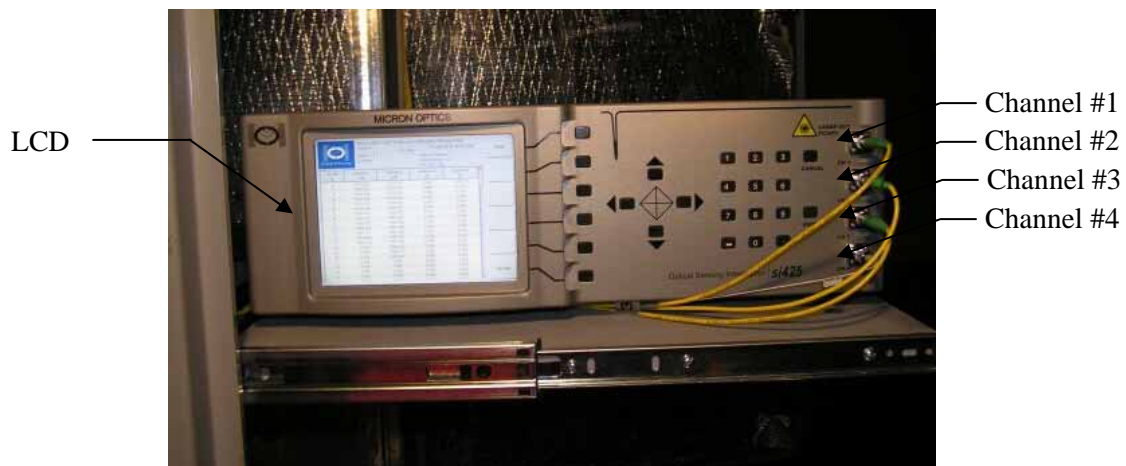
Figure 4.16. Front panel of the Si425-500 interrogator
