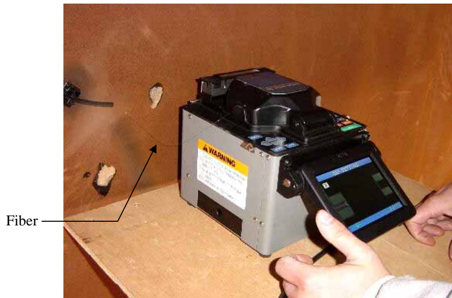
Figure 4.11. Fusion splicing of two fibers
