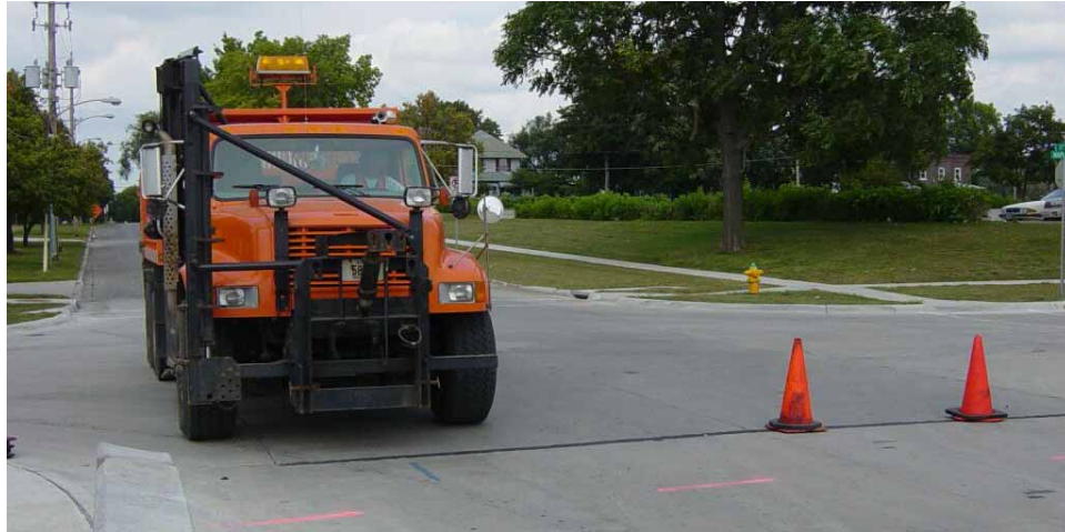
a. Load truck prior to controlled load test
