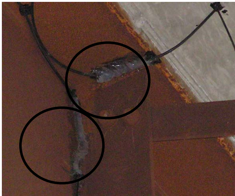
b. Typical web gap sensor (lower circle) and flange tipping sensor (upper circle)
