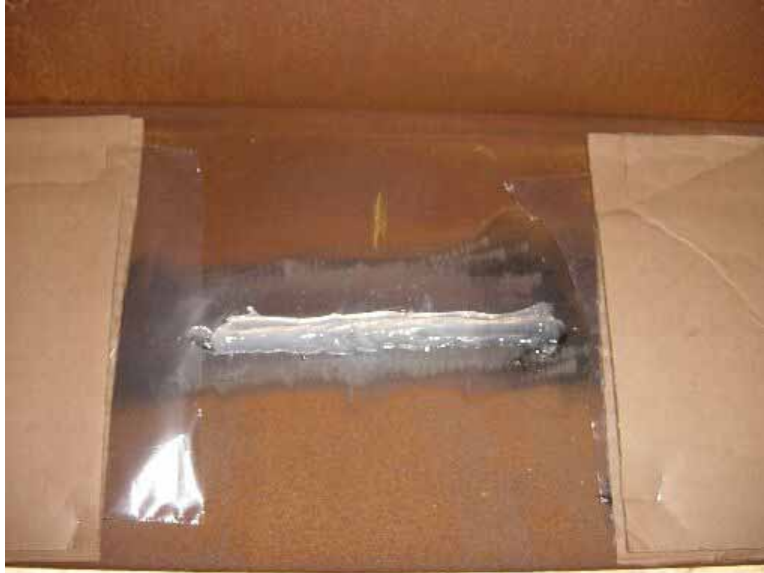
Figure 4.14. Sensor covered in silicone
