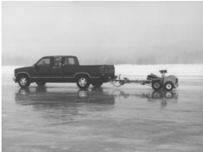
FIGURE 4.8 RUNAR friction trailer.
