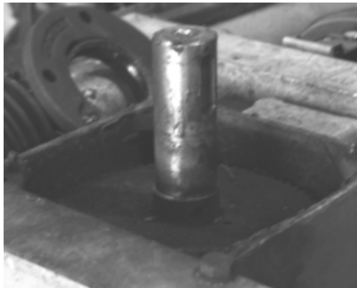
FIGURE 4.23 Shaft with some corrosion.
