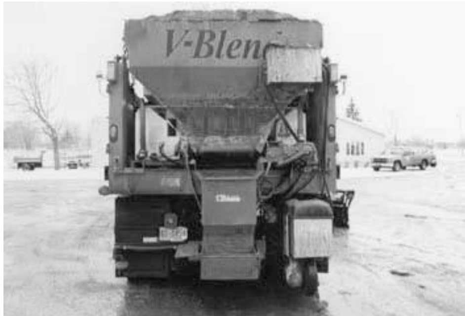
FIGURE 1.2 Tyler V-blend, dual-chamber V-box spreader on Minnesota vehicle.
