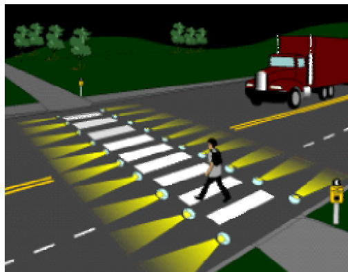
Figure 1. In-pavement flashing warning lights (walkinginfo.org)
