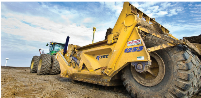
Figure 4-5. A scraper equipped with AMG technology.
