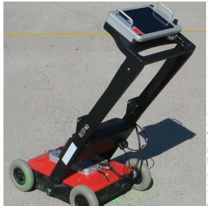
Figure 2-24. Walk-behind ground penetrating radar system.
