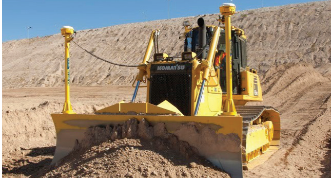
Figure 4-4. A dozer equipped with AMG technology.
