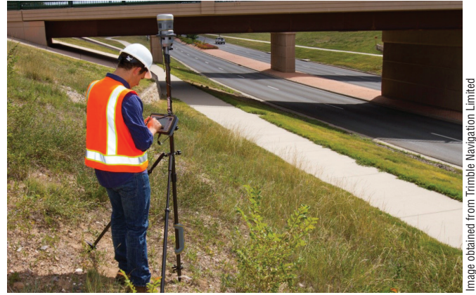
Figure 4-21. Construction inspectors can use survey-grade GPS rovers to traverse the site and spot check elevations.
