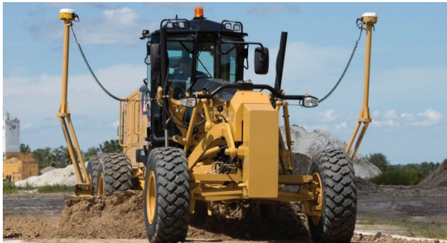
Figure 4-3. A motor grader equipped with AMG technology.
