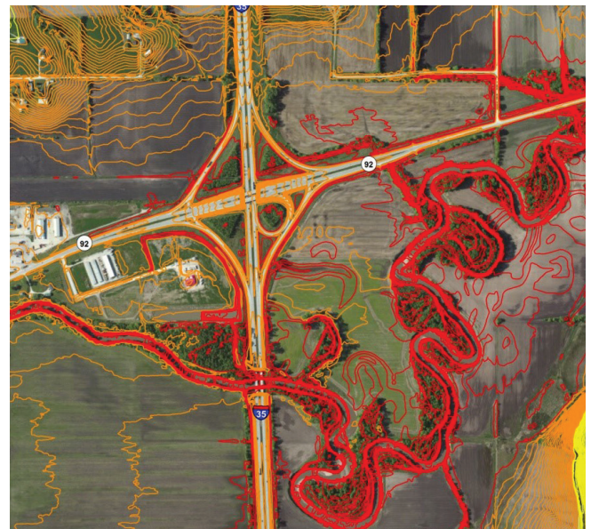
Figure 3-2. Elevation contours created using aerial LiDAR data.
