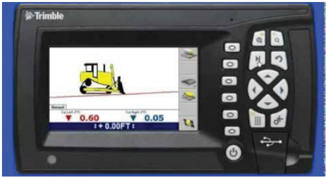
Figure 4-2. Example of a monitor inside the cab of a dozer equipped with AMG technology.
