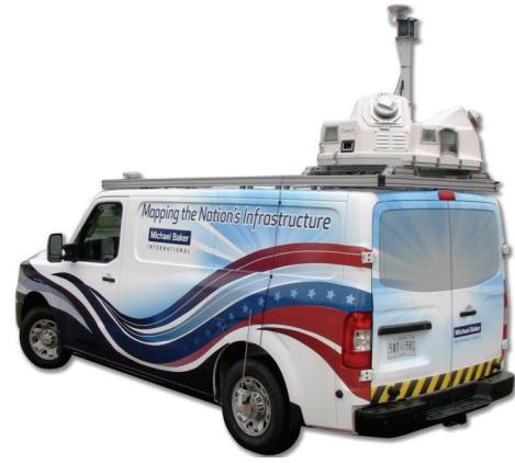
Figure 2-14. Mobile LiDAR vehicle used for obtaining survey data.
