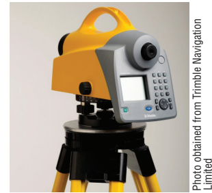
Figure 2-10. Digital level used for transferring elevations across a project site.
