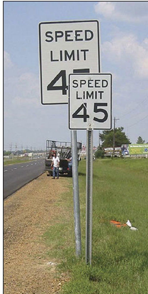
Figure 7. Mississippi DOT upgrades of sign size (Image source: MDOT from Amparano and Morena 2006)
