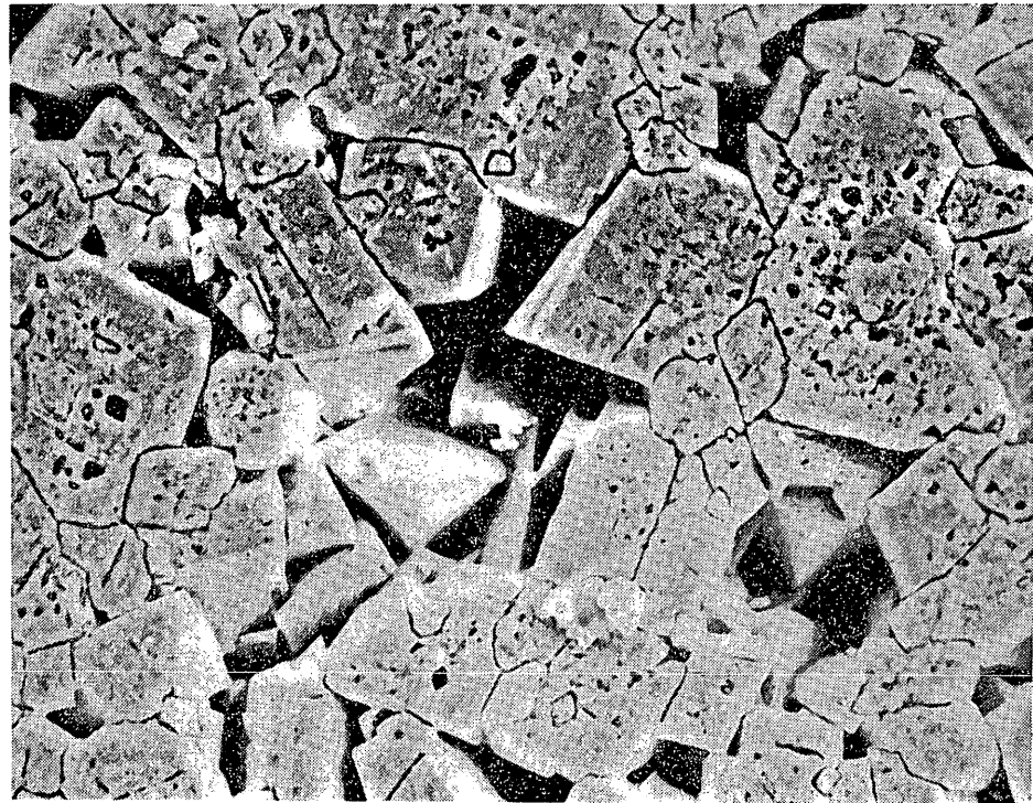
Figure 4 SEM photomicrograph of a polished Garrison dolomite surface after boiling in a sodium chloride solution
