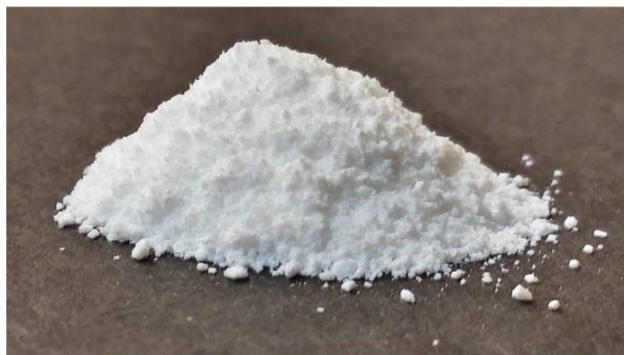
Figure 8 Mg-Al double-layered hydroxides with chloride as exchange anion with best molar ratio (DLHCL31100).
