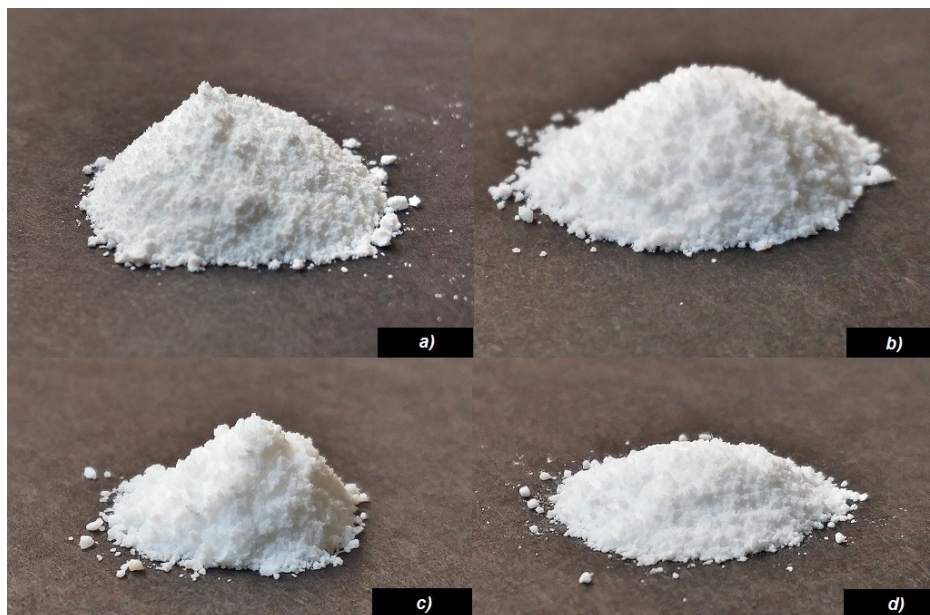
Figure 7 Mg-Al double-layered hydroxides with carbonate as exchanging anion with four different molar ratios. a) DLH1100, b) DLH21100, c) DLH31100, and d) DLH41100.
