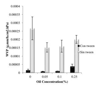
**Graphic 4** Water vapor permeability in chitosan films with essential oil of Cymbopogon citratus at concentrations of 0, 0.05, 0.1 and 0.25 of EO with and without Tween. a-b
