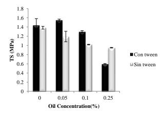
**Graphic 3** Tensile Strength on films of chitosan with essential oil of Cymbopogon citratus at concentrations of 0, 0.05, 0.1 and 0.25 of EO with and without Tween. a-c
