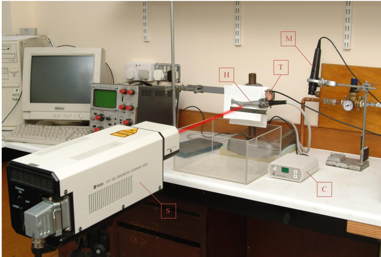
Figure 6.2: Arrangement of equipment for unloaded measurements. The path of the laser beam is indicated by a red line. The beam is directed from the scanning head of the vibrometer (S), toward the vibrating handpiece (H). In this example, a speed-increasing handpiece is being regulated by a table-top control unit (C), and the metal coil transducer (T) is acting as the reference signal. The nearby microphone (M) is for use with turbine handpieces, and would be arranged close to the top of the handpiece head.
