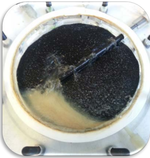
Figure S2: Photographs of both carbon felt (a) and Berl saddles (b) anodes at the end of the experiments.
