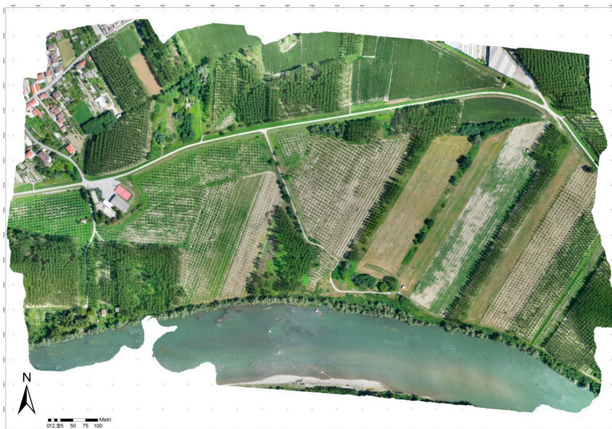
Figure 11. Orthophoto based on the images acquired with the fixed-wing UAV (direct georeferencing approach).
