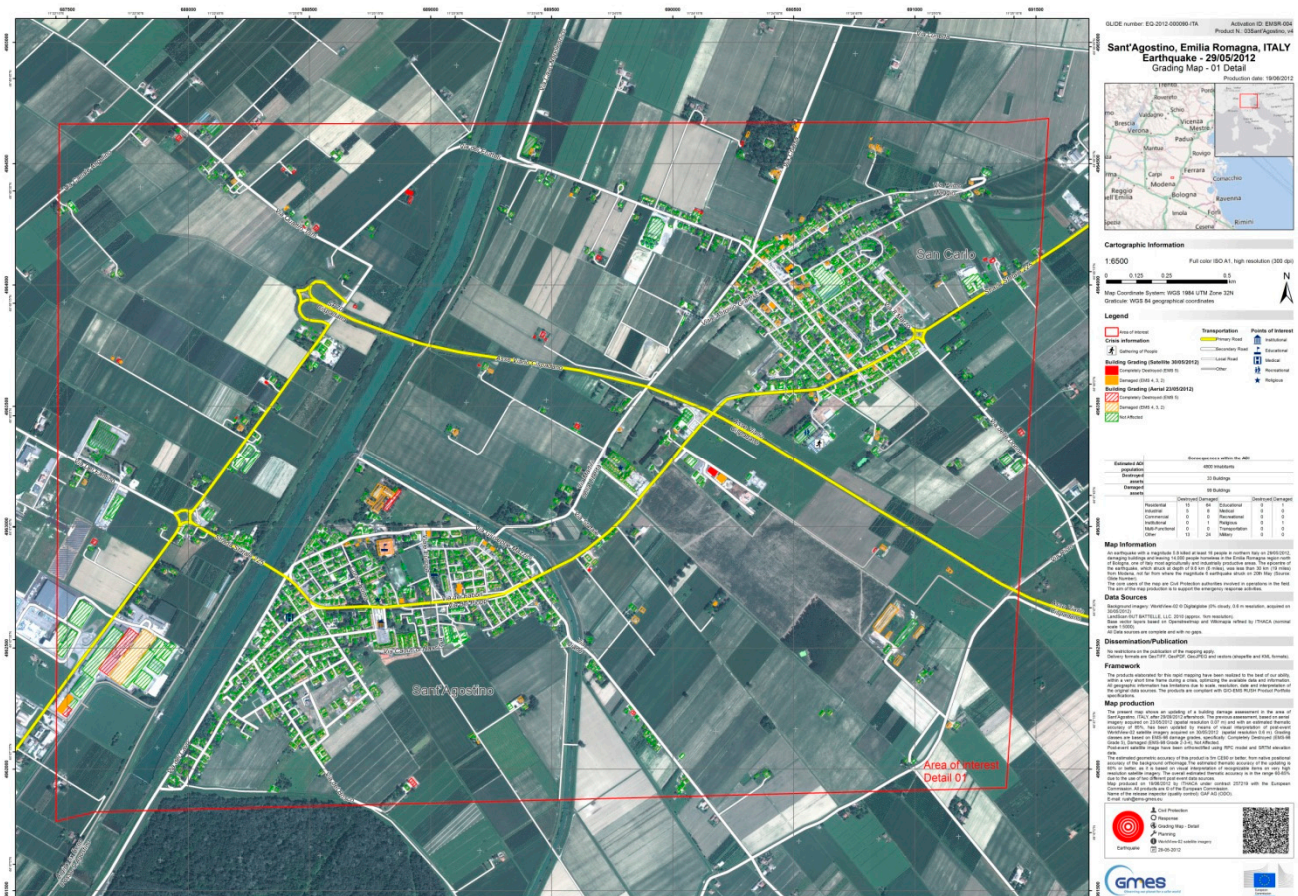
Figure 12. Example of post-event damage assessment map based on both aerial and satellite imagery (Copernicus Emergency Management Service–Mapping [26]).
