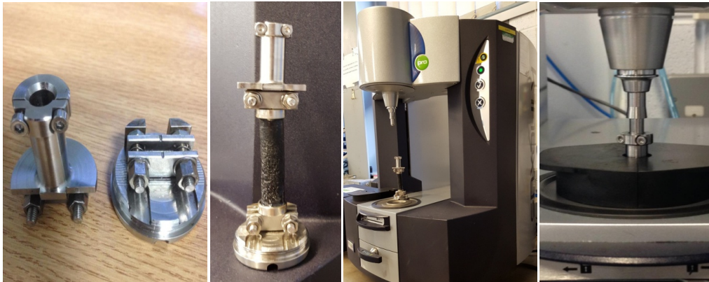
Figure 6.28 Mortar samples installation.
