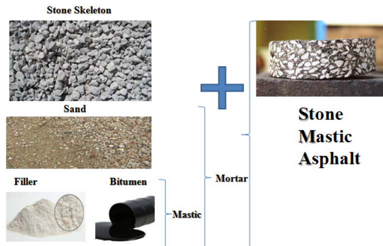
Figure 2.9 Stone Mastic Asphalt composition
