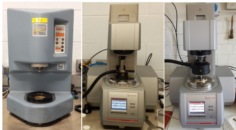
Figure 6.6 DSR used: a) Bohlin - Gemini 200 b) Anton Paar – Smart Pave 102 c) Anton Paar – Smart Paar – MCR 302
