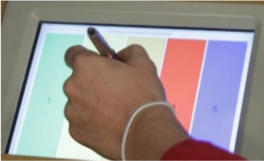
Figure 26. The ISA test is typically presented to the participants in the form of a colour-coded keypad. The keypad flashes and sounds when the workload rating is required, and the participant simply pushes the button that corresponds to their perception of workload.
