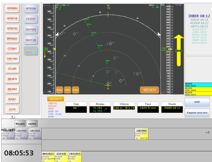
Figure 22. The interface of the Pseudo Pilots provided information about all the airplanes on the RADAR and those assumed by the ATCOs. Furthermore, the Pseudo Pilots could modify the airplane upset depending on the ATCOs instructions or intentionally to produce particular events (e.g. conflicts).
