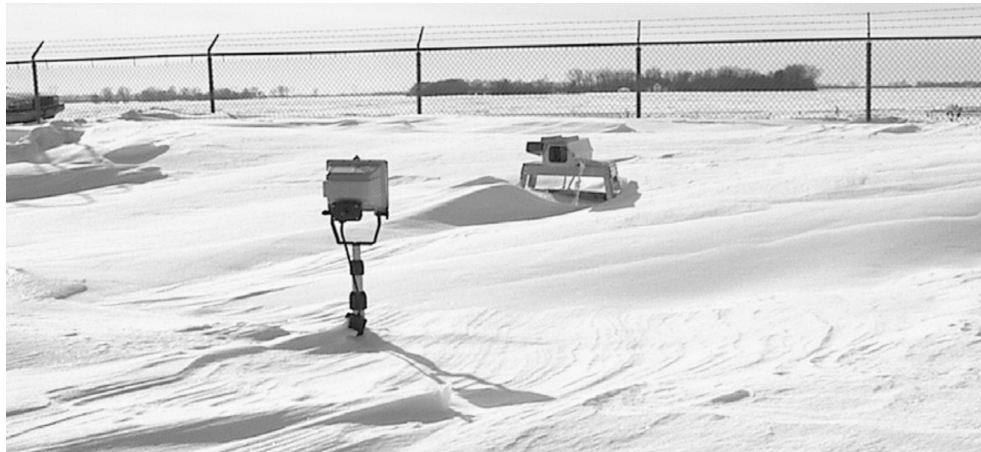
Fig. 5.4 PIP instrument installation. The camera is located in the heated housing on the right of the image, while the lamp is on the left. Image taken from Newman and Kucera (2009)
