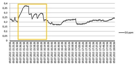
Figure 3.5. Time course of DO in the tank during the production process, measured in the specula with the fluorescent dot.
