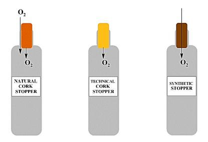
**Figure 2.12.** Schematic representation of mechanisms of oxygen permeation in wines after bottling, when using different closures; the scheme is inspired by previous studies on permeation of wine closures to oxygen (Lopes et al., 2007).
