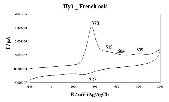
**Figure 6.1.** Cyclic voltammograms (background subtracted) of a French oak tannin (sample Hy3) in model wine solution, measured at 100 mV s<sup>-1</sup> above the potential range: -200 to 1000 mV, at a 3 mm glassy carbon electrode.
