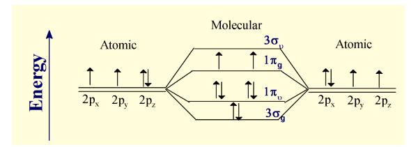
Figure 2.4. Schematic representation of the outer molecular orbitals of the paramagnetic <sup>3</sup>O<sub>2</sub> molecule.
