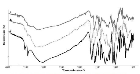
Fig. 3. ATR FT-IR spectra of the most common monomeric units of tannins. (a) (+)-catechin; (b) gallic acid; (c) ellagic acid.
