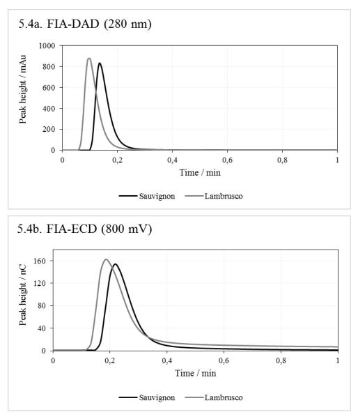
**Figure 5.4.** FIA-DAD (5.4a) and FIA-ECD (5.4b) experiments performed on a white wine (Sauvignon Blanc) and a red wine (Lambrusco). The same injection was used for subsequent analyses, following reequilibration of both detection systems. Peak areas were then calculated to calibrate the response in mmol GAE  $L^{-1}$ .
