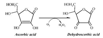
Figure 2.8. Oxidation route of ascorbic acid in oenological conditions.
