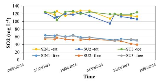
**Figure 4.5**. Evolution of free and total SO<sub>2</sub> parameters for the three series in 9 months of bottle storage. SU2 series (natural cork) underwent the most significant decrease in both parameters.
