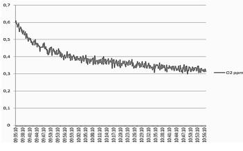
Figure 3.7. Route of the dissolved oxygen during transport as monitored by the PSt3 sensor.
