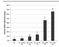
Fig. 1 Antioxidant activity of polymers expressed as percent ABTS radical scavenging for ethyl cellulose (*EC*) films with different additions of grape tannin (*GT*). *Bars* not connected by the *same letter* are significantly different (p < 0.01)
