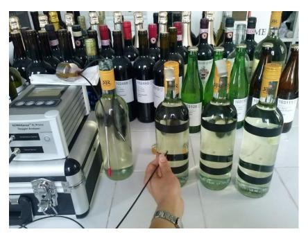
Figure 2.12. The measurement of dissolved oxygen with the colorimetric method after Nomacorc (Limbourg-Dolhain, France).
