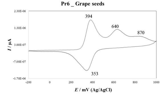
**Figure 6.2.** Cyclic voltammograms (background subtracted) of a grape seed tannin (sample Pr6) in model wine solution, measured at 100 mV s<sup>-1</sup> above the potential range: -200 to 1000 mV, at a 3 mm glassy carbon electrode.
