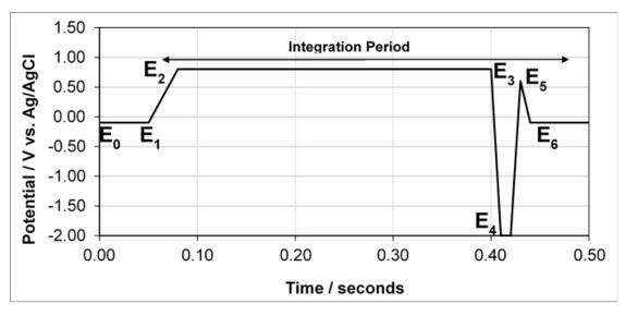
**Figure 5.3.** Integrated amperometry waveform used to determine the antioxidant activity of phenolic compounds in wines and model wine solutions. Detector response is the charge from integration of the phenolics oxidation current between 0.20 and 0.50 s, expressed as nC.
