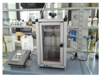
Figure 2.14. The sampling chamber to measure dissolved oxygen in bottled wines after AntonPaar (Graz, Austria).
