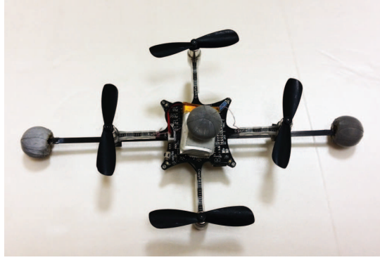
Figure 6.18: Crazyflie quadrotor with structure and markers
