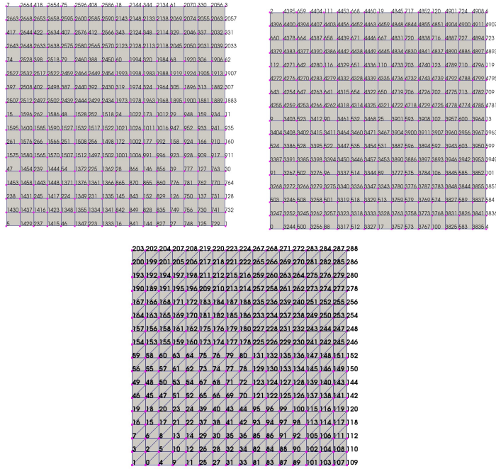
Figure 2.13: Example 2. Numbering of the same surface in MEDmesh (bottom) and in MGMTes as \Omega_1 (left top) and as \Omega_2 (right top).
