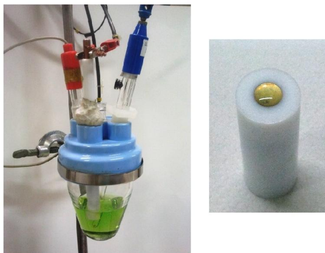
Figure 6.1 – Left: image of the electrochemical cell during the Ni/Fe LDH electrodeposition, right: Pt electrode coated with an electrochemically synthesized Ni/Fe LDH film.
