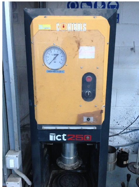
Fig. 5.15: gyratory compactor used for the present research
