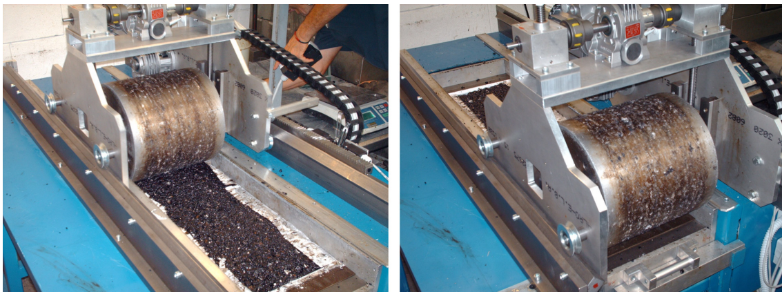
Fig. 3.15: compaction of an asphalt slab with the Elletipi roller compactor
