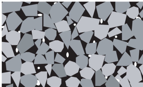
Fig. 3.6: schematic representation of voids in a reference volume of asphalt mixture. White areas represent the air voids, black and white areas represent the VMA
