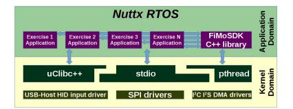
Figure 4.2: Software Architecture.
