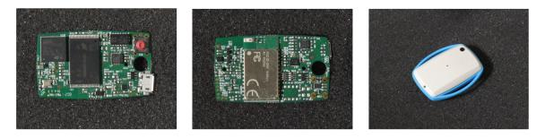
Figure 2.2: The EXLs1 sensing unit.
