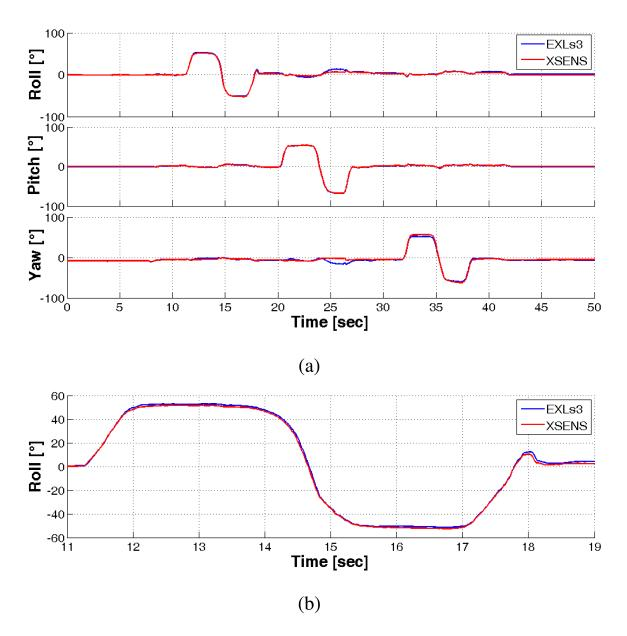
Figure 2.3: (a) Comparison of orientation estimation as computed by Xsens MTw (red) and EXLs1 (blue) sensor nodes using the Kalman filter. (b) Zoom of the roll plot.
