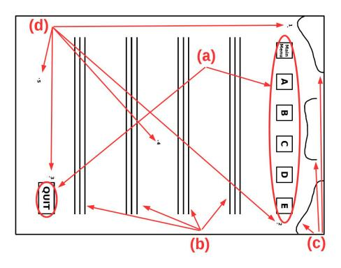
Figure 4.3: Paper User Interface elements layout. a) Menu Buttons; b) Exercise rows; c) Pen Receiver suggested positions; d) Calibration points.
