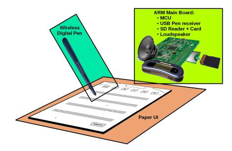
Figure 4.1: Hardware Setup.
