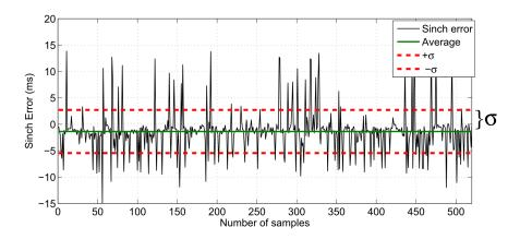
Figure 3.11: Synchronization error after correcting the Bluetooth clock value
