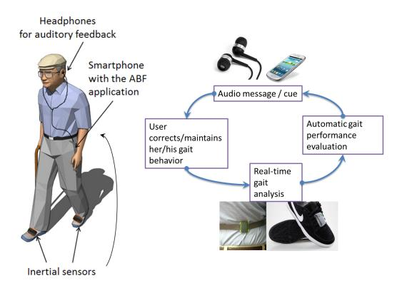
Figure 2.1: Scheme of the scenario for the use and the components of the system
