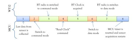
Figure 3.9: Sequence of operation performed during to read piconet clock
