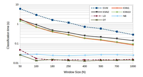
Figure 6.1: Execution time for different classifiers, compared with same training set (referred to an array of 1000 instances)
