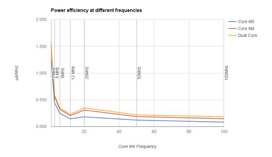
Figure 8.3: Power Efficiency at different operating frequencies (lower is better)
