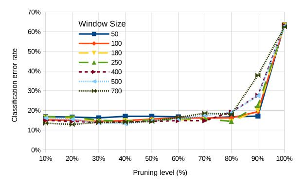
Figure 6.5: Classification error rate on multiple subject with different pruning levels
