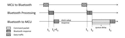
Figure 3.10: Description of how the "read clock" command is processed by a Bluetooth module [RR07]
