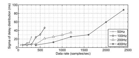
Figure 3.7: Synchronization measurement results, data rate is dependent from sampling frequency and number of nodes connected
