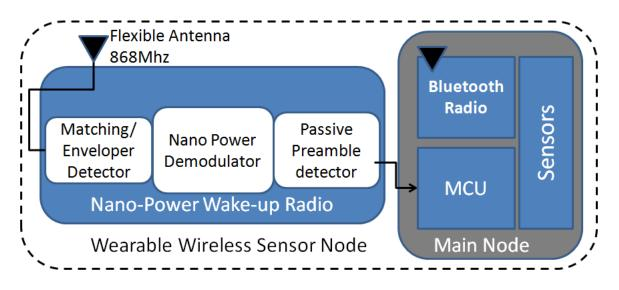
Figure 7.1: Wearable Wireless Sensor Node Architecture.
