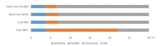
Figure 8.9: Duty cycle of the various core when processing at 30Hz
