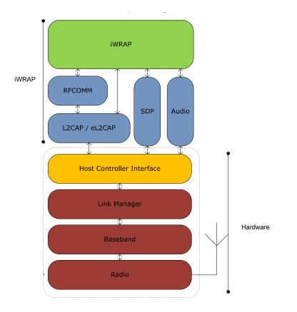
Figure 3.8: Bluetooth stack implemented in WT12 modules
