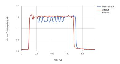
Figure 8.5: Current consumption for the Sensor communication task using DMA and polling almost the same energy consumption. We measured 3.380 mJ using DMA and 3.383 mJ using polling.
