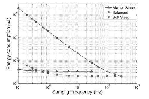
Figure 3.4: MCU Power consumption per cycle
