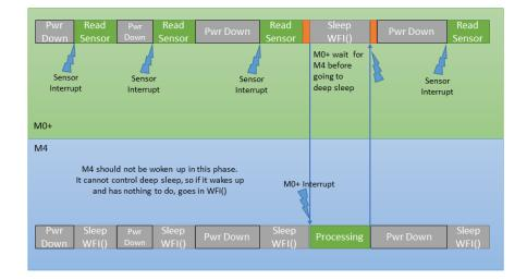
Figure 8.6: Dual core serial implementation time diagram
