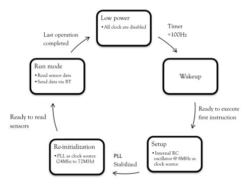
Figure 3.3: State machine for low power modes
