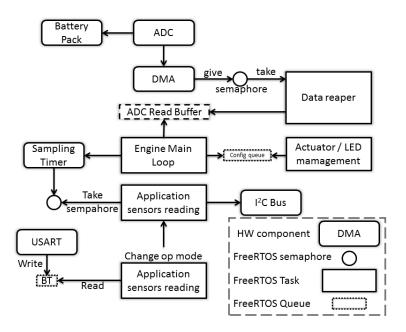
Figure 5.3: FreeRTOS system architecture for Cupid node implementation.
