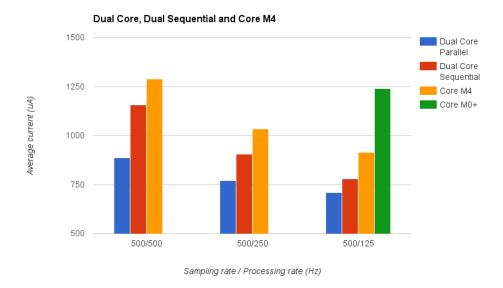
Figure 8.10: Average current consumption for the filtering application, in this case the core M0+ was able to process only 1 sample every 4 new data (sampling rate 500Hz, processing rate 125Hz)
