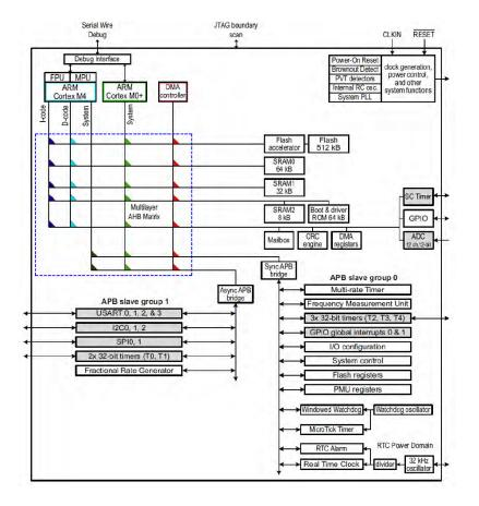
Figure 8.1: Advanced Hugh Performance Bus multilayer matrix for the LPC54102
