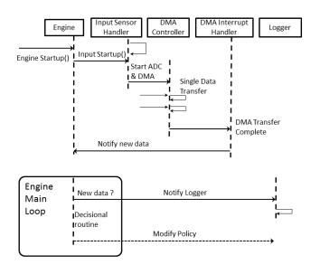
Figure 5.2: DMA input and data transfer for EBM
