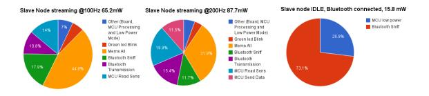
Figure 7.3: Slave node power consumption breakdown for different configurations.
