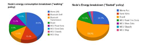
Figure 6.3: Node's power consumption breakdown
