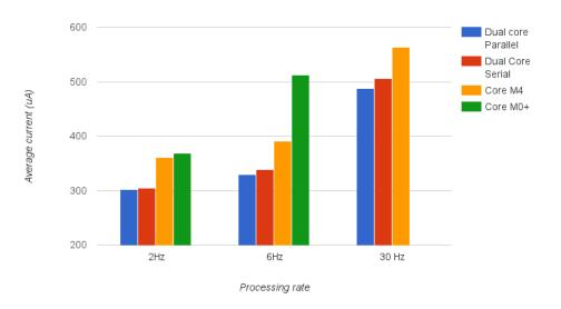
Figure 8.8: Comparison of the average current consumption for different processing rates. M0+ did not complete the computation on time for the 30Hz processing rate
