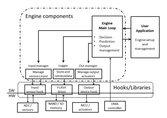
Figure 5.1: EMB Architectural overview. The engine components interact with hardware by means of libraries and application provided hooks. Hooks themselves can rely upon hardware abstraction libraries.
