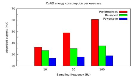
Figure 5.4: Power consumption for different use cases scenarios and battery levels, as the battery level decrease, sampling rate is reduced; use case activity control the policy (Performance, Balance, and Powersave).
