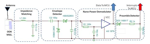
Figure 7.2: Wake up radio diagram.
