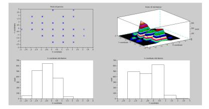
Figure 4.6: The Staedtler Digital pen 990 distibution of the coordinates of the pen tip held still caused by noise.
