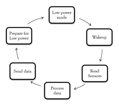
Figure 3.1: State machine for typical WBAN node
