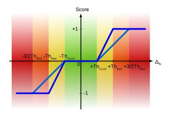
Figure 4.4: Score relative to the difference between measured value and TargetValue.  $Th_{Bad}$  and  $3/2 * Th_{Bad}$  are used depending on the application state.
