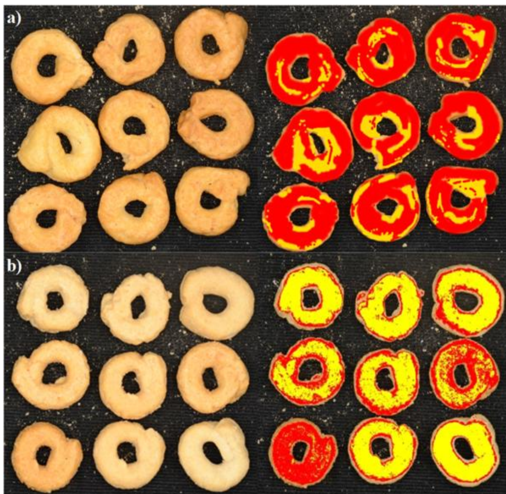
Fig. 3 Taralli images and virtually coloured samples on the basis of different levels of browning area calculated with advanced image analysis software. Dark area, virtual colour red (a), light area, virtual colour yellow (b)
