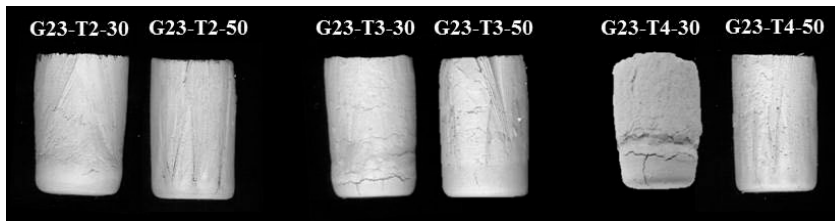
Figure 4.9 Freeze-cast monoliths ( \varnothing=15\text{mm} , h=25\text{mm} ) obtained applying maturation step T2, T3 and T4 and adding 30 and 50 vol.% of water.
