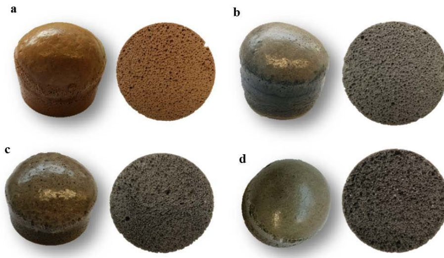
Figure 6.15 Expanded structure and core section of the selected foams: a) M4-Na, b) M1-K, c) Fds-Na, and d) Fds-K.
