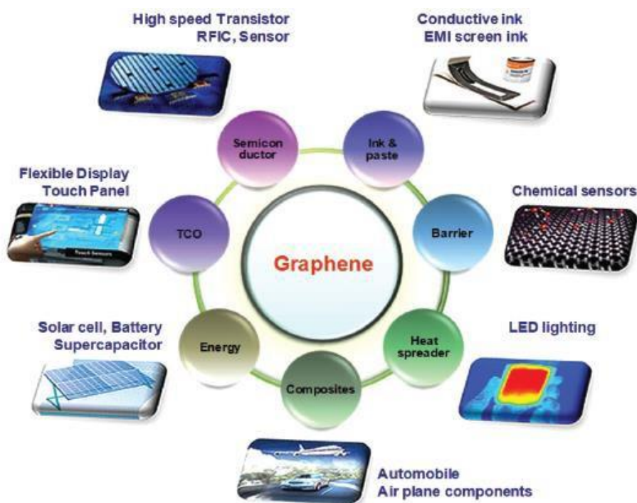
Fig. 7: Overview of applications of Graphene in different sectors ranging from conductive ink to chemical sensors, light emitting devices, composite materials, energy, touch panels and high frequency electronics[8].
