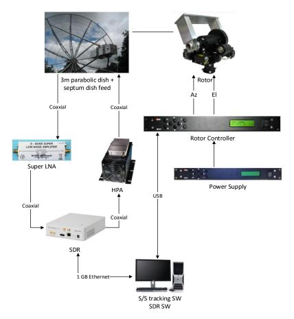
Figure 23. S-band ground station
