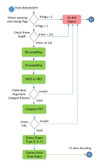
Figure 7. Bit operations and frame detection (downlink)
