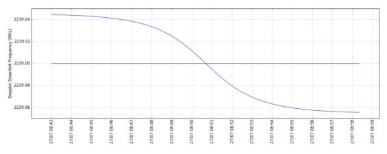
Figure 78. Doppler corrected downlink frequency for Metop-A pass over CDA1, orbit 45500
