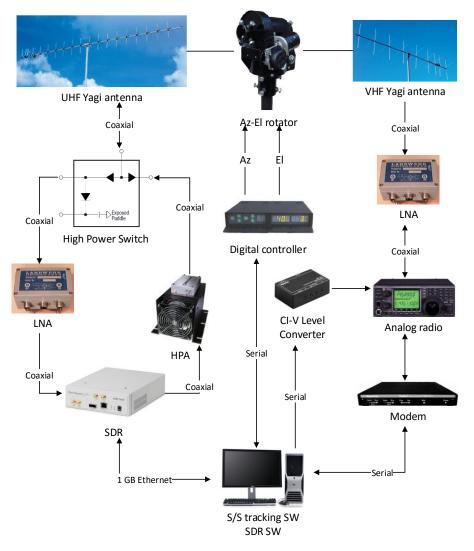
Figure 22. VHF/UHF ground station
