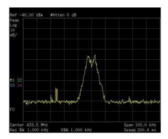
Figure 31. GFSK signal spectrum
