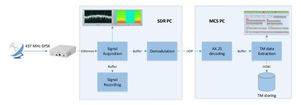
Figure 38. Downlink chain flowchart
