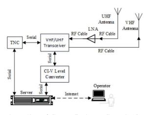
Figure 13. Forlì Ground Station configuration for ALMASat-1 mission
