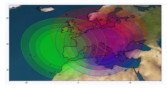
Figure 10. Detail of the visibility circles of Forlì, Munich and Vigo stations (5°, 10°, 15° and 20° minimum elevations)
