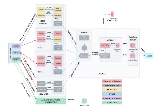
Figure 12. ESEO Ground Segment detailed block diagram
