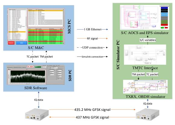
Figure 43. S/C simulator block diagram
