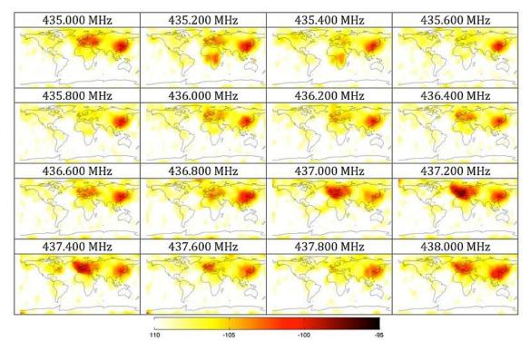
Figure 8. RSSI (dBm) average interference world plot between 6/8/2014 and 11/8/2014
