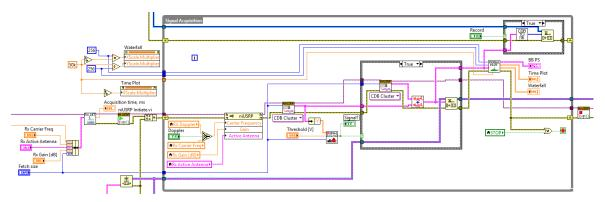
Figure 26. LabVIEW block diagram of the signal acquisition loop of the SDR software
