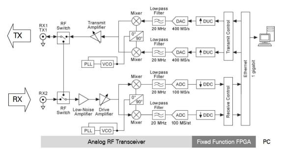
Figure 21. USRP block diagram
