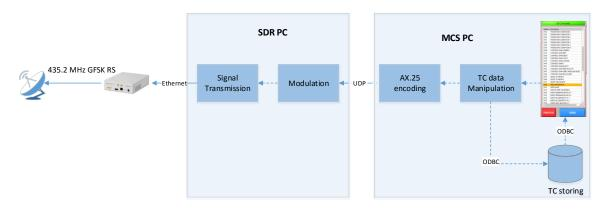
Figure 37. Uplink chain flowchart
