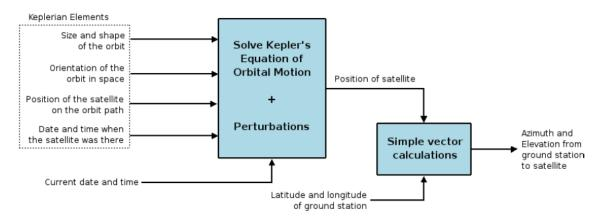
Figure 24. Computation of azimuth and elevation from ground station to satellite
