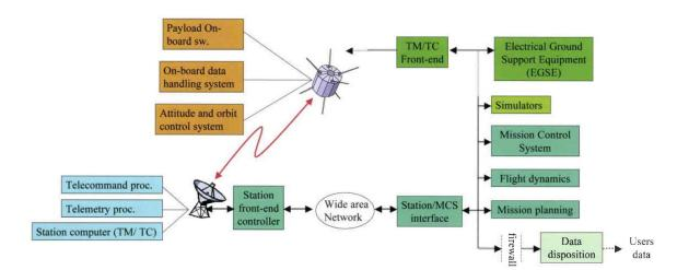
Figure 1. Schematic of typical space system, with the emphasis on software elements [1]
