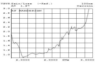
Figure 16. VSWR plot for the RX port of the septum dish feed by RF Hamdesign
