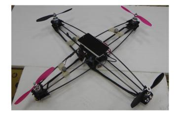
Figure 4.1: The quadrotor prototype
