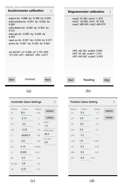
Figure 4.10: Auxiliary activities: (a) Accelerometer calibration (b) Magnetometer calibration (c) Set Controller gains (d) Set position gains
