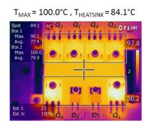
c) IR picture of the Si prototype at output power of 2000 W.
