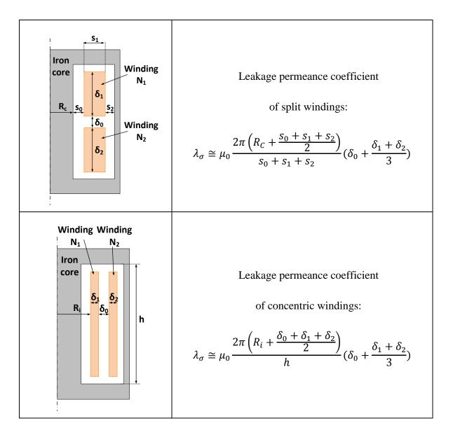
Table 3.4 - Leakage permeance coefficients of split and concentric windings.
