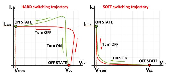
Figure 2.6 – Comparison of hard and soft switching trajectories.
