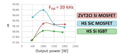
Figure 3.57 - Efficiency of prototypes as a function of output power at a switching frequency of 20 kHz.
