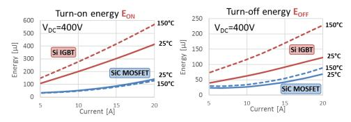
Figure 3.54 – Switching energies of the Si IGBT and SiC MOSFET selected.
