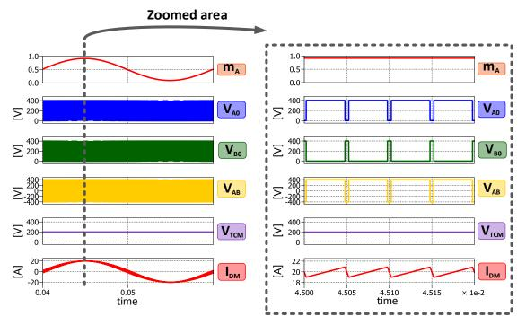
Figure 4.13 – Simulation results of full bridge converter controlled by means of bipolar modulation.
