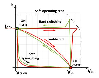
Figure 3.1 – Comparison of typical hard, snubbered and soft switching trajectories of an IGBT or BJT.
