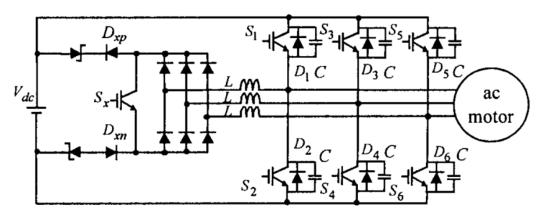
Figure 3.8 - Schematic of a three phase ZVTSS.
