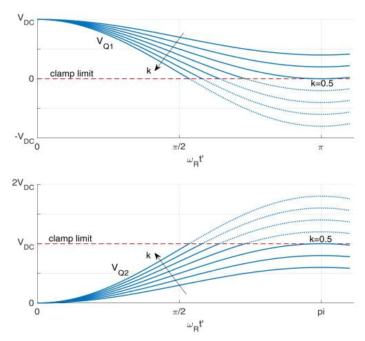
Figure 3.21 – Resonant transition of voltages  $V_{Q1}$  and  $V_{Q2}$  during time [t<sub>2</sub>, t<sub>3</sub>].
