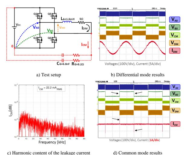
Figure 4.38 - Experimental results of full bridge converter controlled by means of hybrid modulation.
