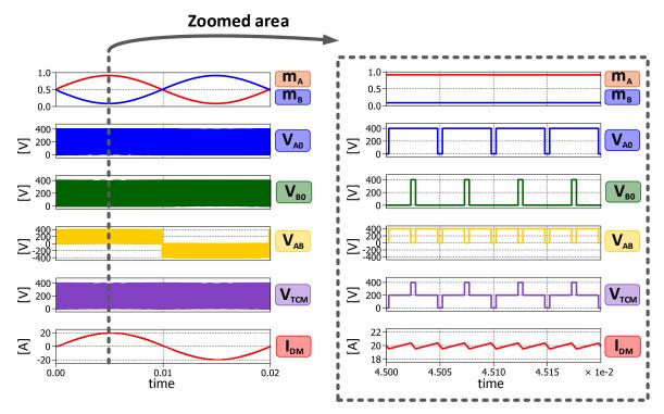
Figure 4.15 - Simulation results of full bridge converter controlled by means of unipolar modulation.
