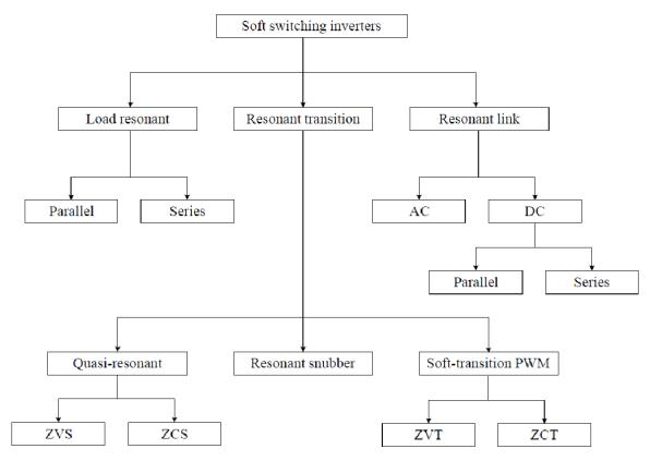
Figure 3.2 - Classification of soft switching DC/AC converters
