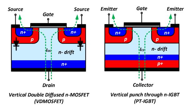
Figure 1.7 – Comparison of the structure of a VDMOSFET and of a PT IGBT.
