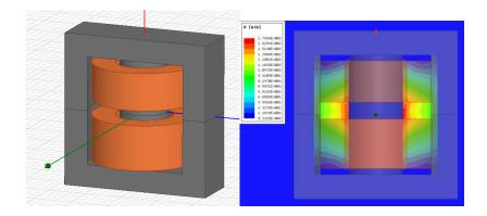
Figure 3.43 – Detail of the FEA model of the autotransformer.
