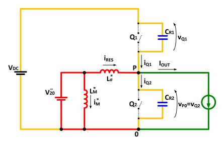
Figure 3.19 - Equivalent circuit of the ZVT2CI converter during time [t<sub>2</sub>, t<sub>3</sub>].
