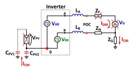
Figure 4.7 – Simplified model of the PV system.
