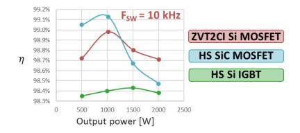
Figure 3.56 – Efficiency of prototypes as a function of output power at a switching frequency of 10 kHz.
