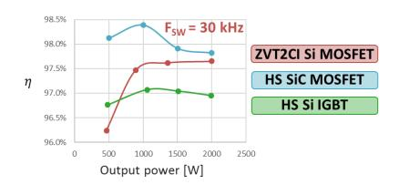
Figure 3.58 - Efficiency of prototypes as a function of output power at a switching frequency of 30 kHz.
