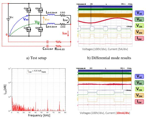
c) Harmonic content of the leakage current
