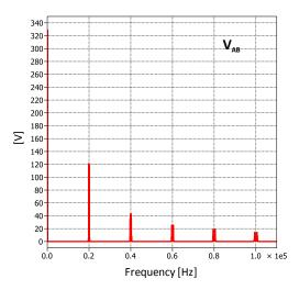
Figure 4.18 - Harmonic content of the output voltage  $V_{AB}$  generated by low side discontinuous modulation.
