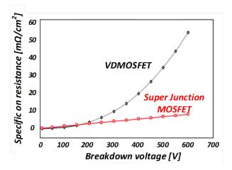
Figure 1.6 – 1D-Silicon limits of VDMOSFETs and SJ MOSFETs
