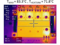
c) IR picture of the Si prototype at output power of 2000 W.
