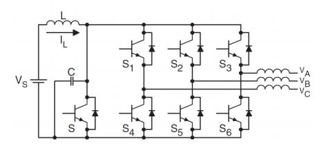
Figure 3.3 - Resonant DC-Link Inverter.
