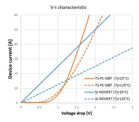
Figure 2.1 – V-I characteristic two typical 650 V IGBT and SJ MOSFET rated for the same current
