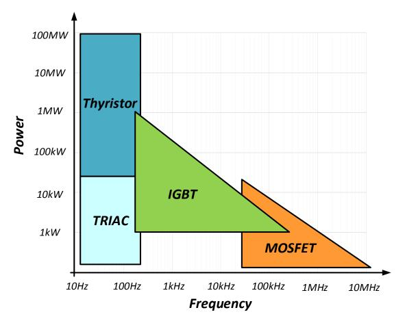
Figure 1.1 - Application of discrete power semiconductors.
