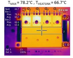
c) IR picture of the Si prototype at output power of 2000 W.
