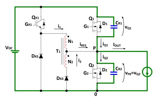
Figure 3.30 - Detail of the ZVT2CI converter during time [t<sub>7</sub>, t<sub>8</sub>].
