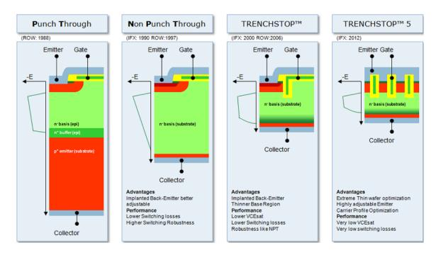
Figure 1.8 - Evolution of Infineon IGBTs, from Punch Trough to TRENCHSTOP™ 5 technology
