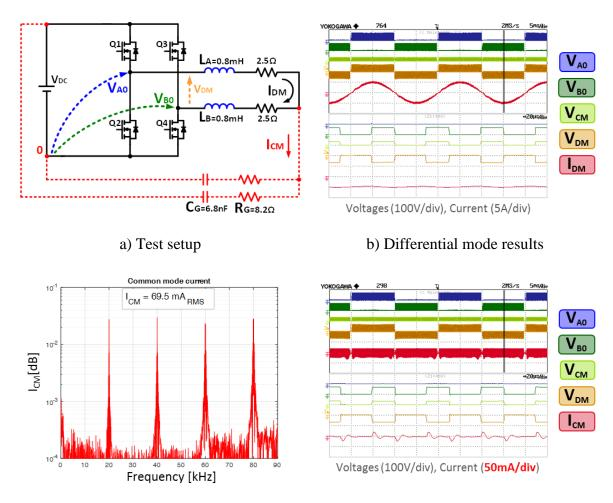
c) Harmonic content of the leakage current
