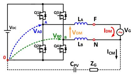
Figure 4.12 – Grid connected full bridge converter.
