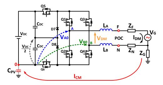
Figure 4.26 - Grid connected H6 converter.
