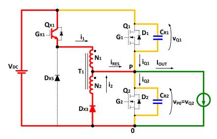
Figure 3.18 - Detail of the ZVT2CI converter during time [t<sub>2</sub>, t<sub>3</sub>].
