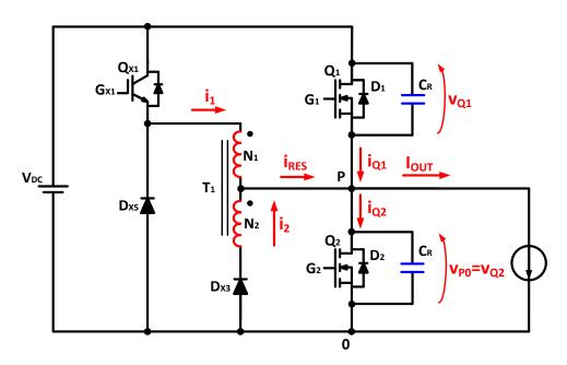
Figure 3.13 - Schematic of the ZVT2CI converter, considering only the main bridge and the positive current auxiliary pole.
