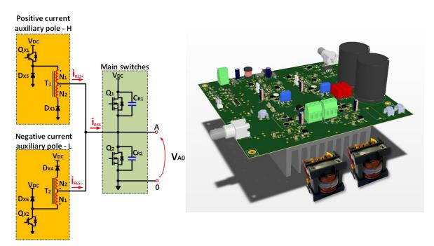
Figure 3.45 – Schematic and 3D rendering of the prototype of ZVT2CI converter.
