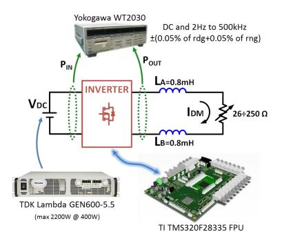
Figure 4.45 – Experimental test setup.
