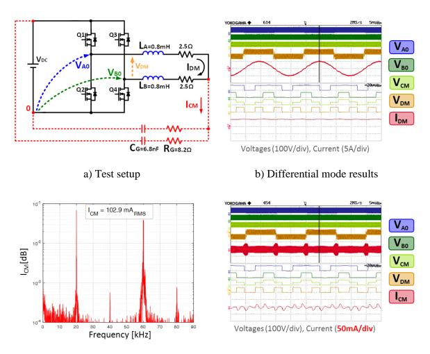
c) Harmonic content of the leakage current
