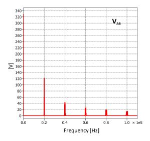
Figure 4.24 - Simulation results of H5 converter controlled by means of high side discontinouos modulation.
