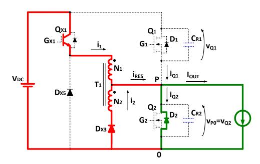
Figure 3.16 - Detail of the ZVT2CI converter during time  $[t_1, t_2]$ .
