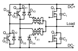
Figure 3.11 - Schematic of a ZVT2CI inverter leg.
