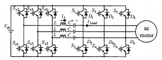
Figure 3.7 – Schematic of a three phase ZCT.
