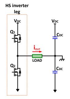
Figure 3.52 - Schematic of a leg of the hard-switching inverter.
