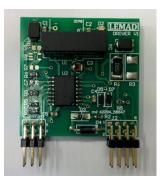
Figure 4.32 – Picture of the gate driver board.
