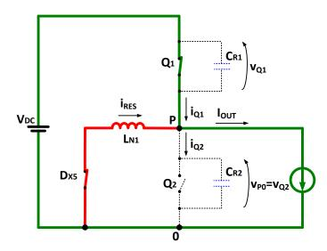
Figure 3.28 - Equivalent circuit of the ZVT2CI converter during time [t<sub>5</sub>, t<sub>6</sub>].
