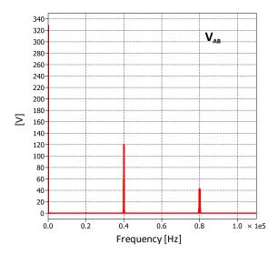
Figure 4.16 - Harmonic content of the output voltage  $V_{AB}$  generated by unipolar modulation.
