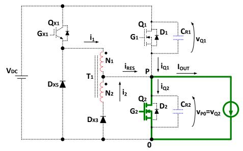
Figure 3.32 - Detail of the ZVT2CI converter during time [t<sub>8</sub>, t<sub>9</sub>].
