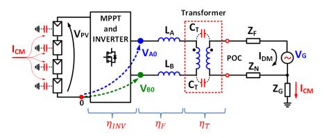
Figure 4.4 – Single phase PV system with isolation transformer.
