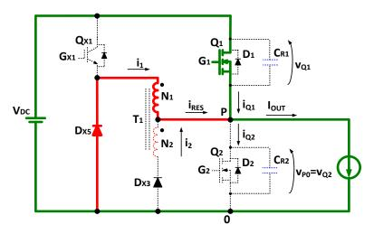
Figure 3.27 - Detail of the ZVT2CI converter during time [t<sub>5</sub>, t<sub>6</sub>].
