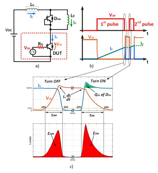
Figure 2.3 – Switching characterization test power switches. a) double pulse tester. b) gateemitter voltage, collector-emitter voltage and collector current of the DUT. c) switching waveforms during turn-on and turn-off.
