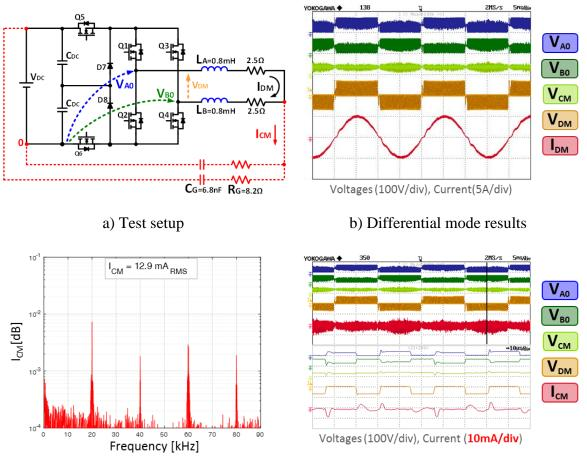
c) Harmonic content of the leakage current
