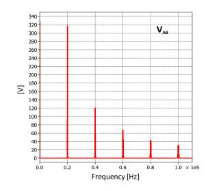
Figure 4.14 – Harmonic content of the output voltage  $V_{AB}$  generated by bipolar modulation.
