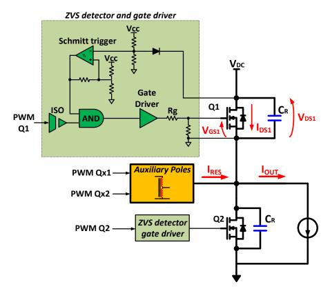
Figure 3.44 – Details of the Zero-voltage detection circuit and gate driver.
