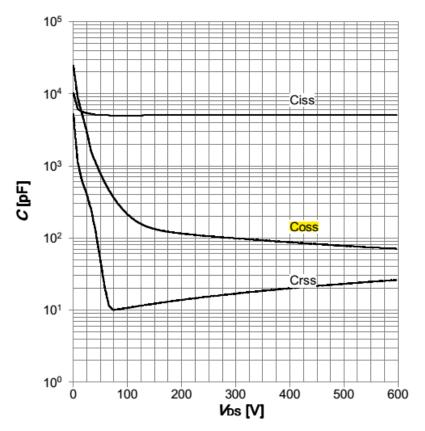
Figure 3.39 - C-V characteristics of IPW65R080CFD super junction MOSFET.
