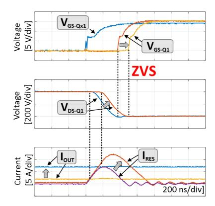
the zero-voltage detection circuit of Figure 3.44 always ensures that  $Q_1$  is turned on only when its drain-source voltage is zero.
