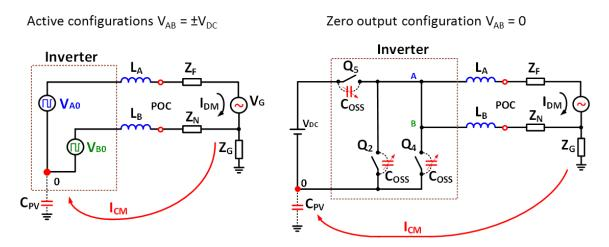
Figure 4.23 – Simplified circuit of the H5 converter during active configurations (left) and zero output configurations (right).
