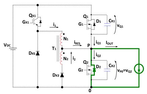
Figure 3.31 - Detail of the ZVT2CI converter during time [t<sub>8</sub>, t<sub>9</sub>].
