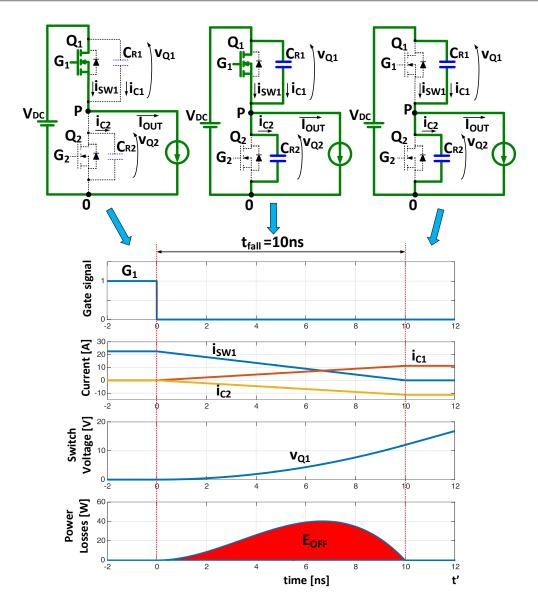
Figure 3.37 - Turn-off loss generation of  $Q_1$  considering a real power transitor.
