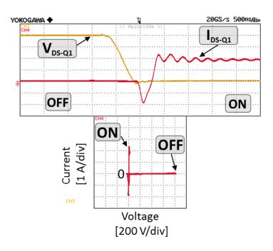
Figure 3.49 - Detail of the zero-voltage turn-on of switch  $Q_1$  and switching trajectory.
