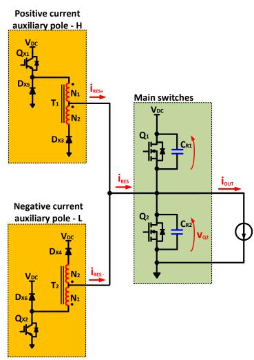
Figure 3.12 - Schematic of a ZVT2CI inverter leg feeding an highly inductive load, approximated by a current source.
