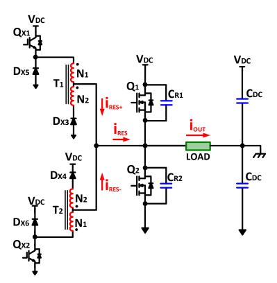
Figure 3.46 - Schematic of a leg of the ZVT2CI inverter.
