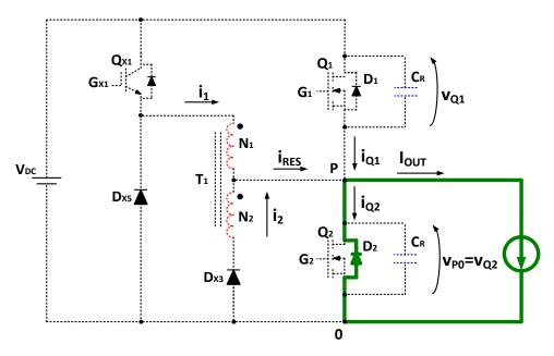
Figure 3.15 – Detail of the ZVT2CI converter during time [t<sub>0</sub>, t<sub>1</sub>].
