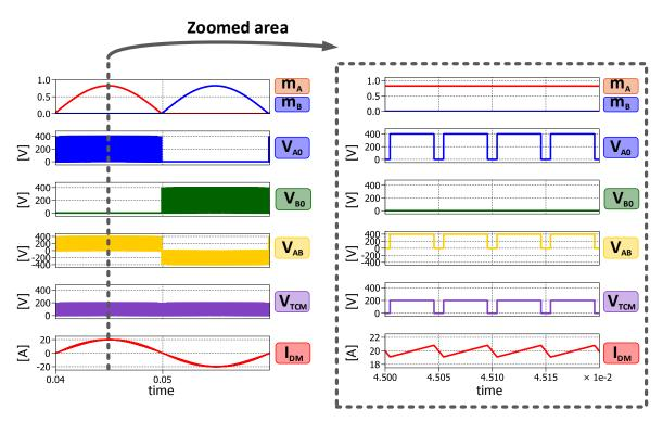
Figure 4.17 - Simulation results of full bridge converter controlled by means of low side discontinuous modulation.
