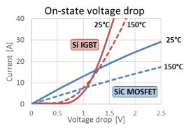
Figure 3.53 – V-I characteristic of the Si IGBT and SiC MOSFET selected.
