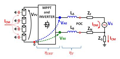
Figure 4.5 - Single phase transformerless PV system.
