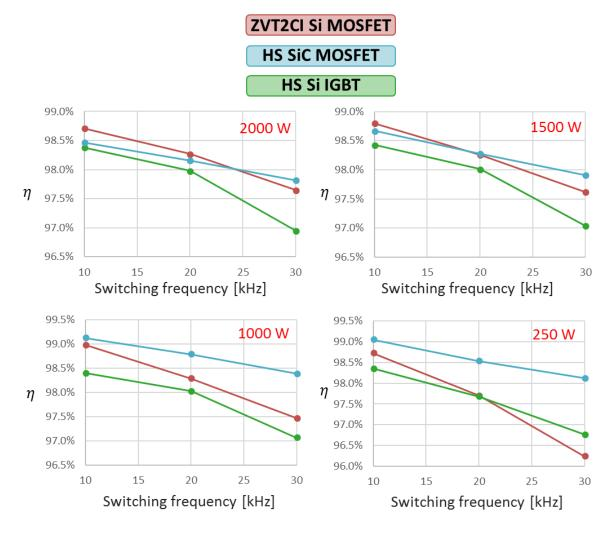
The efficiency of all prototypes is plotted in Figure 3.59 as a function of the switching frequency when the output power is equal to 500 W, 1000 W, 1500 W and 2000 W.
