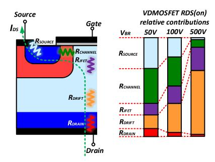
Figure 1.4 - Contribution to the on state resistance of a VDMOSFET as function of the blocking voltage
