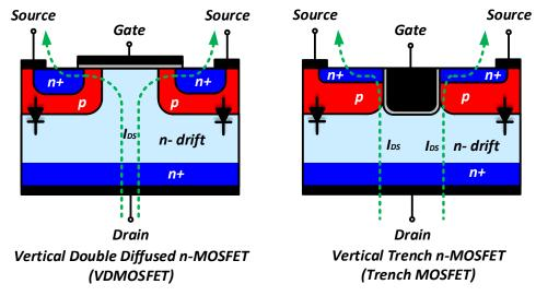
Figure 1.5 – VDMOSFET and trench MOSFET structures.
