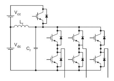
Figure 3.4 - Active-Clamped Resonant DC-Link Inverter.
