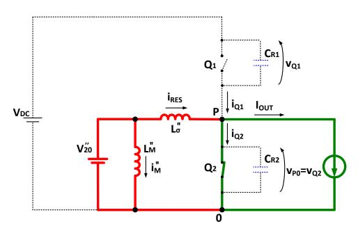
Figure 3.17 - Equivalent circuit of the ZVT2CI converter during time [t<sub>1</sub>, t<sub>2</sub>].
