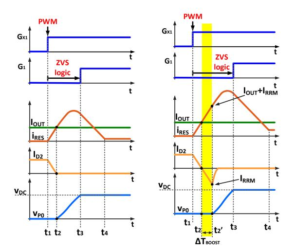
Figure 3.34 - Resonant transition of the converter if ideal diodes are considered.
