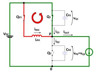
Figure 3.26 - Equivalent circuit of the ZVT2CI converter during time [t<sub>4</sub>, t<sub>5</sub>].
