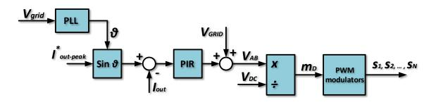
Figure 4.11 - Output current control scheme.
