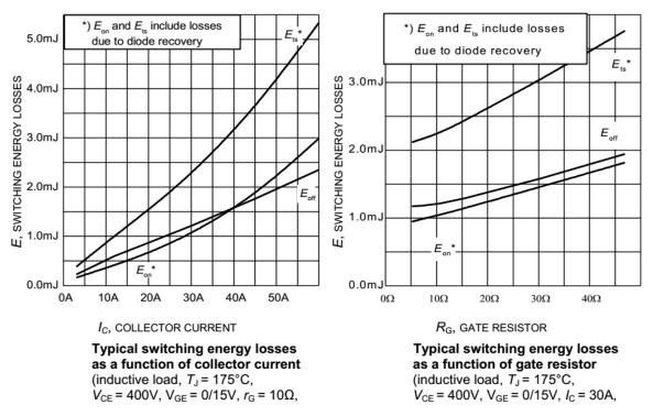
Figure 2.4 – Switching energies of the IGBT Infineon IKW30N60T as function of collector current (left figure) and of gate resistance (right figure)
