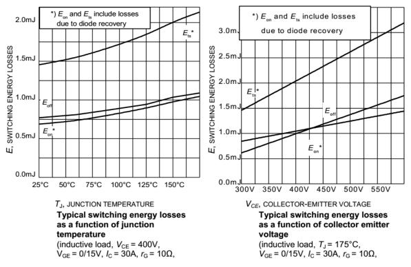
Figure 2.5 - Switching energies of the IGBT Infineon IKW30N60T as function of the junction temperature (left figure) and of collector-emitter voltage (right figure)
