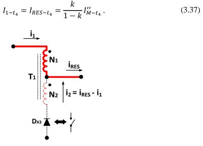
Figure 3.24 – Relation between the resonant current and the currents in the windings of the autotransformer.
