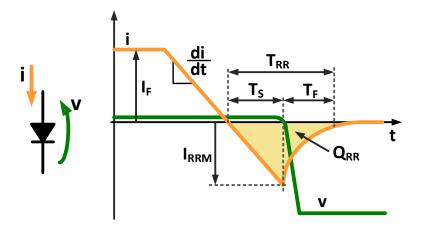
Figure 3.33 - Reverse recovery waveforms and definitions.
