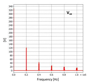
Figure 4.28 - Harmonic content of the output voltage  $V_{AB}$ .
