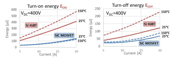
Figure 4.44 – Switching energies of the Si IGBT and SiC MOSFET selected.
