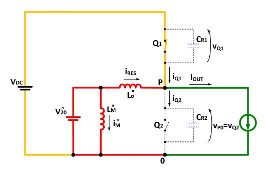
Figure 3.23 - Equivalent circuit of the ZVT2CI converter during time [t<sub>3</sub>, t<sub>4</sub>].
