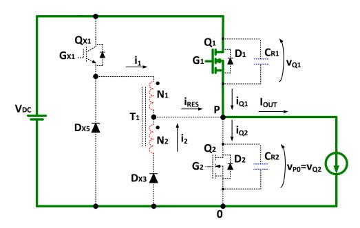
Figure 3.29 - Detail of the ZVT2CI converter during time [t<sub>6</sub>, t<sub>7</sub>].
