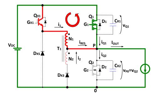
Figure 3.25 - Detail of the ZVT2CI converter during time [t<sub>4</sub>, t<sub>5</sub>].
