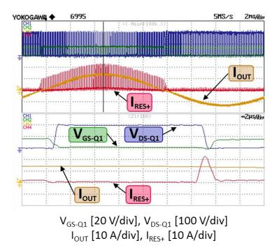
Figure 3.47 - Behavior of the ZVT2CI inverter controlled by means of sinusoidal modulation.
