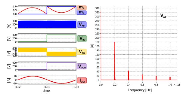
Figure 4.20 - Simulation results and harmonic content of the output voltage  $V_{AB}$  in case of full bridge converter controlled by means of hybrid modulation.
