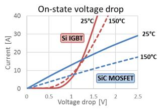
Figure 4.43 - V-I characteristic of the Si IGBT and SiC MOSFET selected.
