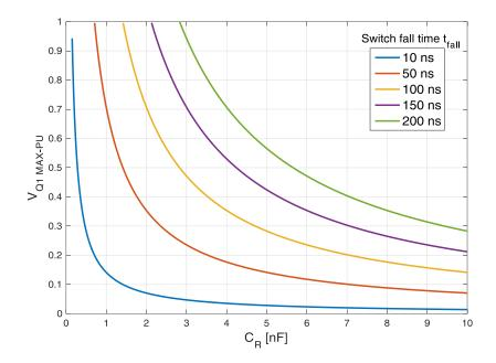
Figure 3.38 – Voltage across switch  $Q_1$  versus snubber capacitor  $C_{R1}$  as a function of the fall time of the transistor. Curves are calculated for a load current of 22.6A.
