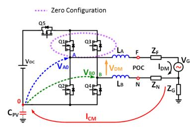
Figure 4.22 - Grid connected H5 converter.
