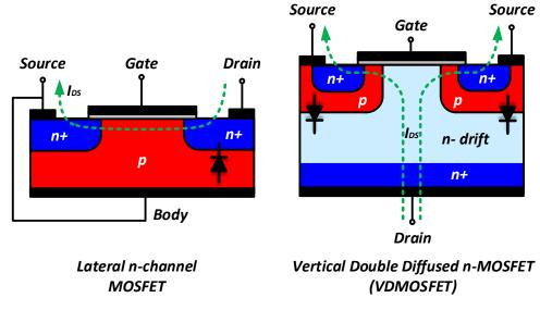
Figure 1.3 – Lateral and vertical MOSFET structures.
