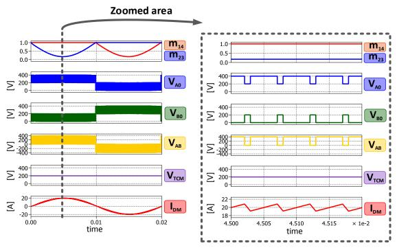
Figure 4.27 - Simulation results of H6 converter.
