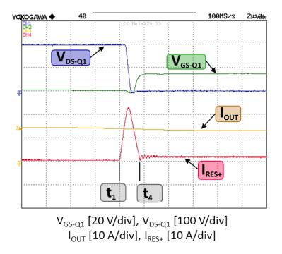
Figure 3.48 – Detail of the zero-voltage turn-on of switch  $Q_1$ .
