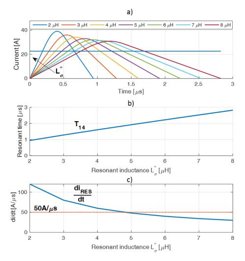
Figure 3.41 - a) Auxiliary current as a function of the leakage inductance of autotransformer. b) Duration of the transition time  $T_{14}$  as a function of the leakage inductance of autotransformer. c) Maximum resonant current variation as a function of the leakage inductance of autotransformer.
