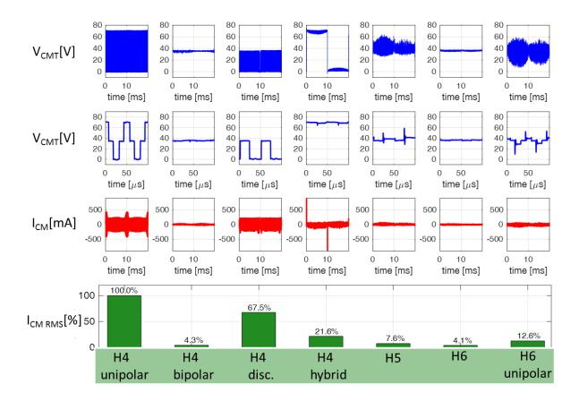
Figure 4.42 – Comparison of the total common mode voltage and leakage current generated by the tested modulation strategies.
