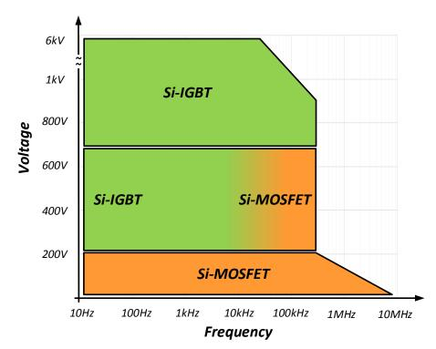
Figure 1.2 - Typical MOSFETs and IGBTs selection as a function of blocking voltage and switching frequency.
