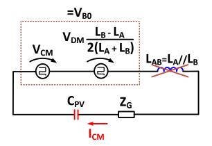
Figure 4.21 – Simplified CM circuit of the full bridge converter controlle by means of hybrid modulation. The total common mode voltage is equal to  $V_{B0}$ .
