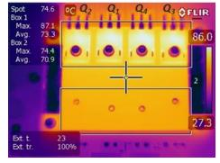
c) IR picture of the Si prototype at output power of 2000 W.
