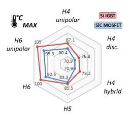
Figure 4.53 – Maximum temperature of the power switches at output power of 2000 W.
