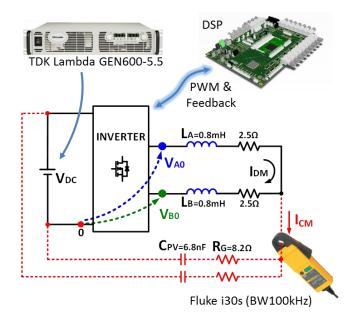
Figure 4.34 – Experimental test setup.
