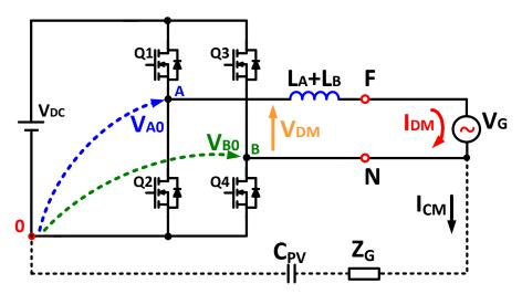
Figure 4.19 - Grid connected full bridge converter controlled by means of hybrid modulation.
