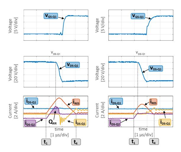
Figure 3.51 – Effect of the reverse recovery of diodes on the behaviour of the converter.
