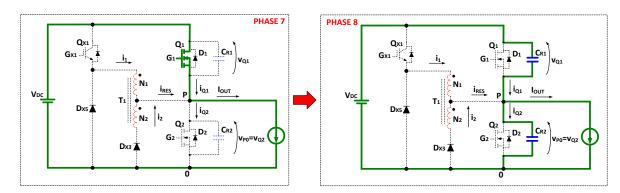
Figure 3.36 – Turn-off of  $Q_1$  considering ideal switches. ZVS is achieved since the load current commutate instantly from the transistor to the capacitor  $C_{R1}$ .
