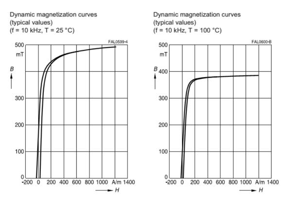
Figure 3.42 – Magnetic hysteresis loop of N87 ferrite.
