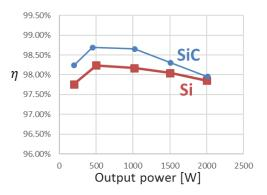
b) Efficiency comparison of SiC and Si prototypes.
