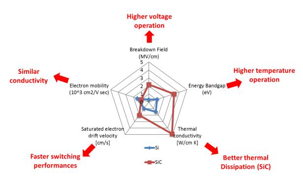
Figure 1.9 - Material properties of silicon and silicon carbide.
