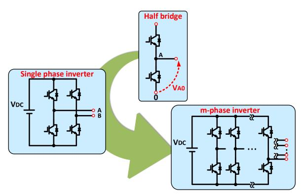
Figure 2.2 – multi phase DC/AC converters based on the half bridge leg.
