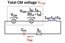
Figure 4.9 - Simplified model of the PV system showing the total common mode voltage  $V_{TCM}$ .
