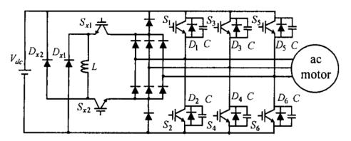
Figure 3.9 - Schematic of a three phase ZVTSI.
