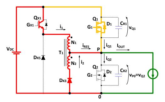
Figure 3.22 – Detail of the ZVT2CI converter during time [t<sub>3</sub>, t<sub>4</sub>].
