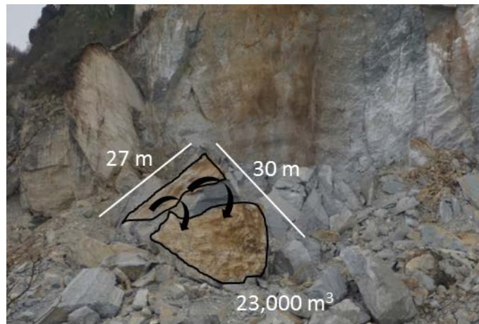
Figure 52. Blocks in the deposit area, which appear to have been broken on impact with the ground
