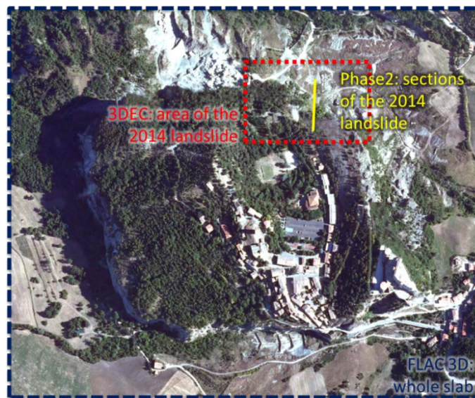
Figure 130. Scales and areas considered in the FLAC3D (blue) 3DEC (red) and Phase2 (green) simulations.
