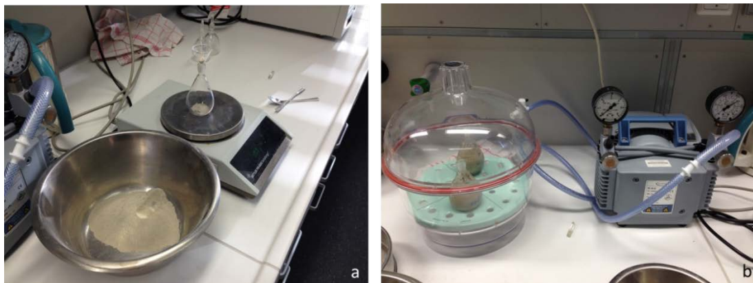
Figure 64. Measure of the specific density: a) pycnometer weighting and b) desiccator
