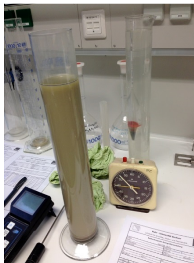
Figure 62. Sedimentation cylinder used for the grain size distribution determination
