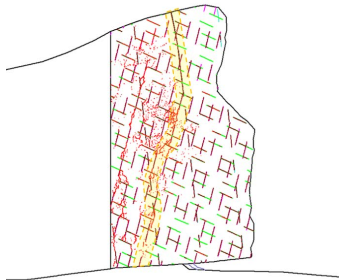
Figure 157. Results of the Voronoi simulation, in red the joints yielded at the failure stage, in dark red the joints yielded at previous stages of the simulation. Non-yielded joints are represented with their original colour (green, magenta and blue), non-yielded Voronoi network is hidden for visualization purposes. The failure surface is highlighted in yellow
