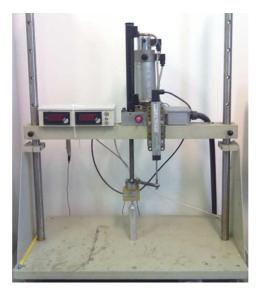
Fig. 43 Compression device with cell of charge of 1 kg.
