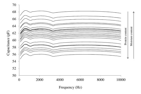
Fig. 27 Average capacitance spectral signals of all the analysed mixtures.
