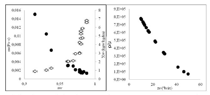
Fig. 13 Physical characterization during the concentration process, the empty dots represent the correlation between **a**w and **x**w; the full dots show the correlation between **a**w and **m**.
