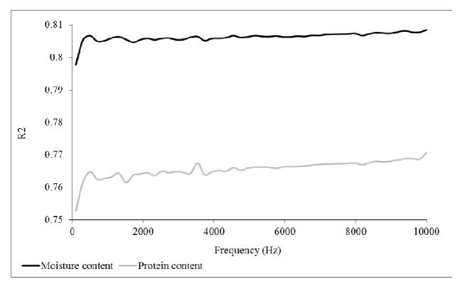
Fig. 28 Trend of the linear correlation between spectral data, protein and moisture.
