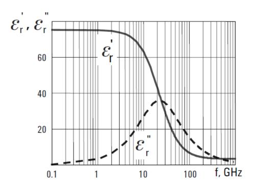
Figure 2 Debye model of the relaxation of water at 30°C.
