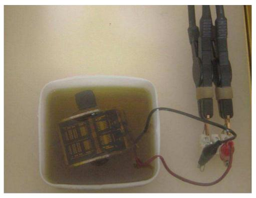
Fig. 5 Parallel plate capacitor covered by EVOO sample.
