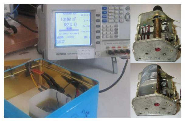
Fig. 4 Instrumental chain and parallel plate capacitor with mobile and fixed plates.
