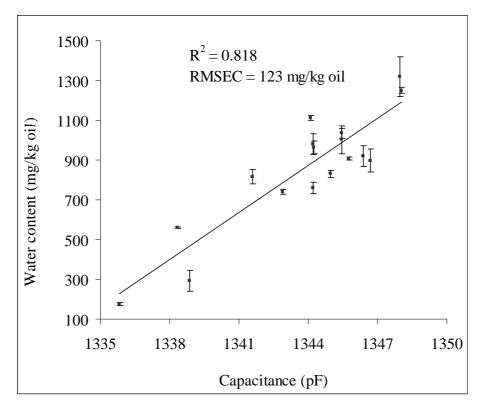
Fig. 7 Correlation between capacitance and water content for all oils at 8 kHz frequency.
