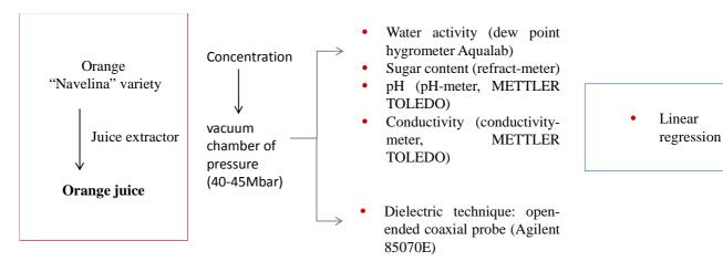
Fig. 12 Experimental plan
