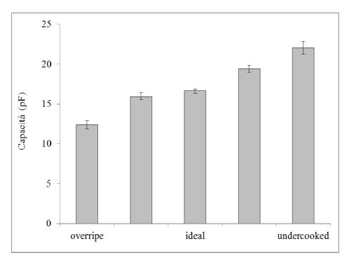
Fig. 47 Capacitance values of five wafer sheets in function of the coking level.
