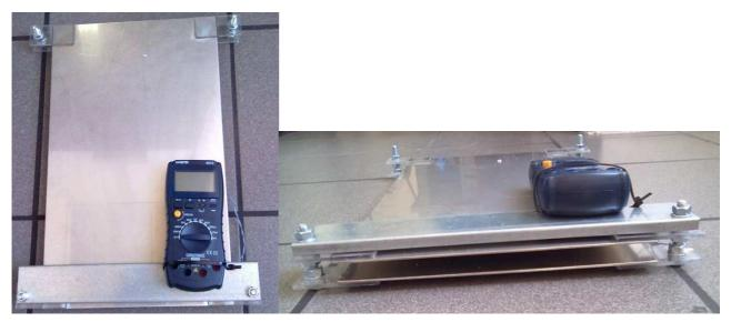
Fig. 42 Parallel plate capacitor
