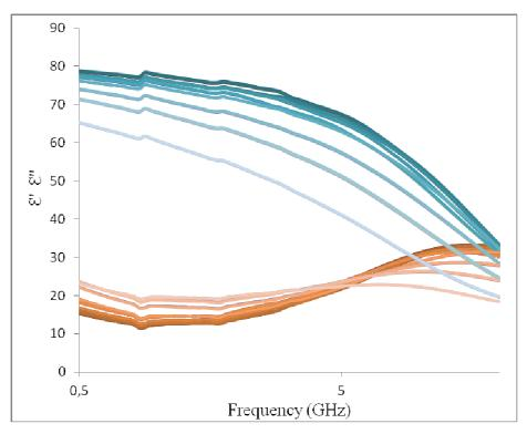
Fig. 15 Dielectric constant and loss factor at different °brix.
