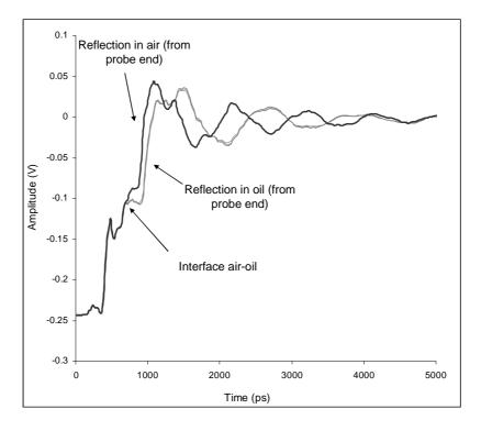
Figure 38. Amplitude (V) of the TDR acquisitions in air and oil.
