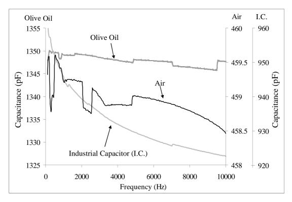
Fig. 11 Capacitance for the probe in air and with an oil having a water content of 1321 mg/Kg oil (n. 12, in Tables 1 and 2), together with an industrial capacitor having a rated capacitance of 1 nF, in the range 100 Hz to 10 kHz.
