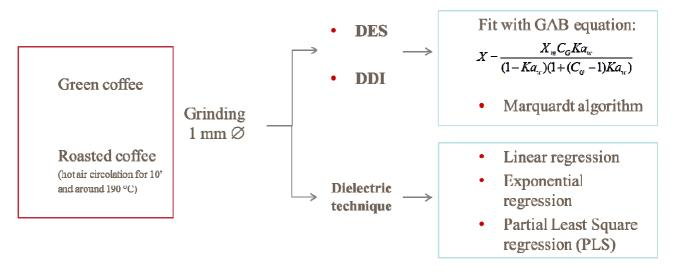
Fig. 17 Experimental plan, DES (Satured salt slurry method) and DDI (Dinamic Dewpoint Isotherm method)
