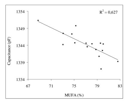
Fig. 10 Correlation between capacitance and monounsaturated fatty acids (MUFA) for all oils at 2 kHz frequency.
