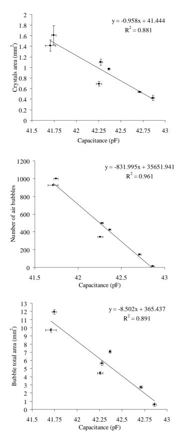
Fig. 37 Correlations between the capacitance and freezing process parameters (with standard error bars).
