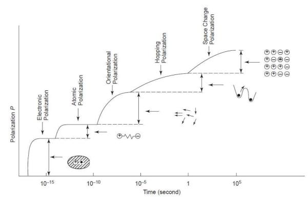
Fig. 1 Polarization effects (de Loor and Meij-boom, 1966).
