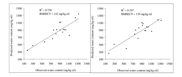
Fig. 8 Predict and observed values for the water content at 2 kHz and 8 KHz (cross validation).
