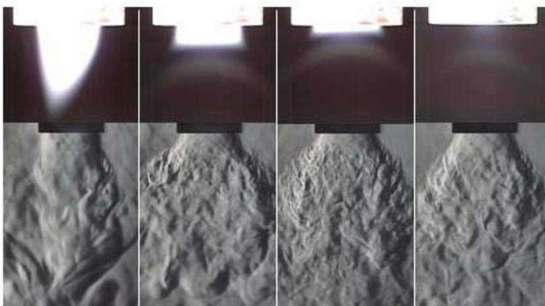
Figure 52. HSI (above) and SI (below) of ICP downstream region in steady conditions with Ar central gas flow rate 0.9 slpm and 500 W: from left to right: sheath gas: Ar 10-16-18 slpm; Ar 14 slpm + air 0.2 slpm; [11] © 2014 IEEE
