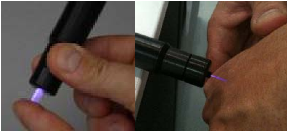
Figure.58 Nanosecond pulsed plasma jet operating in Ar (left) and He (right) [18]
