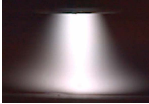
Figure 16 Picture of the operating plasma arc welding process at 70 A. [27]
