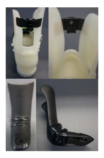
Figure 3.4: Insert and tongues used to modify the stiffness in the 3-pieces ski boot
