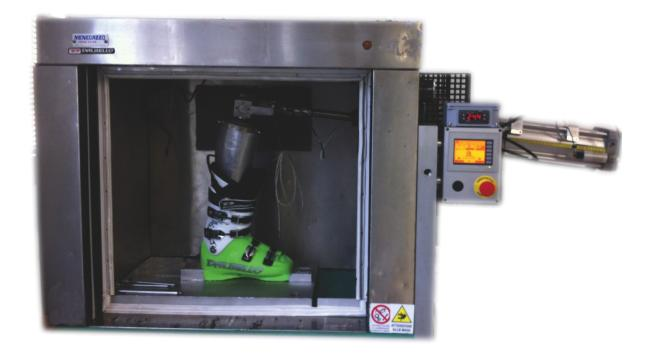
Figure 3.6: Ski boot flexural test bench
