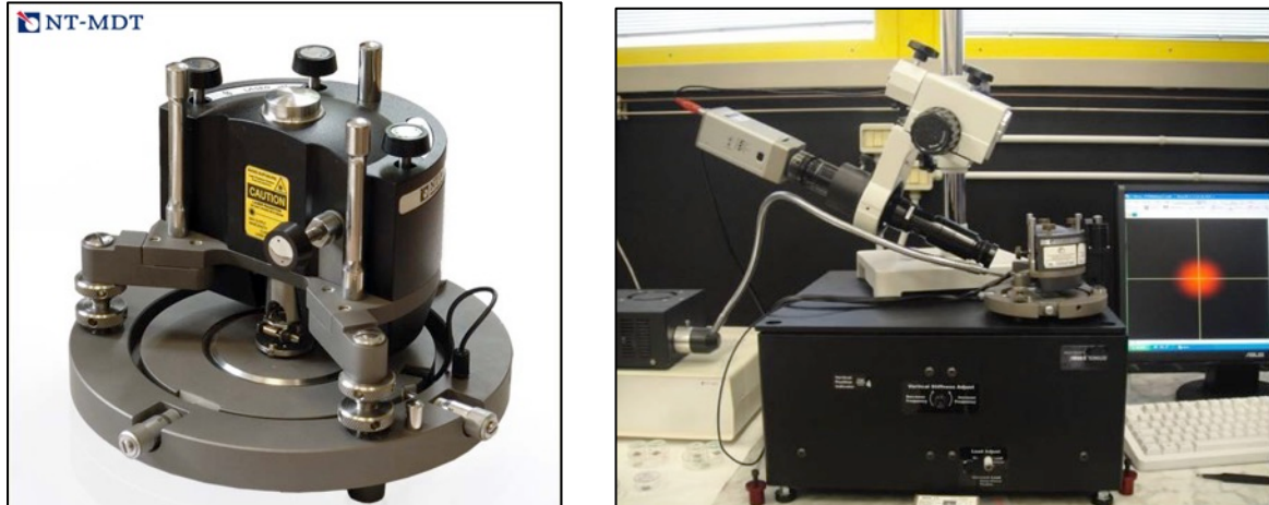
Figure 2.12: a) NT-MDTM Smena Standalone head, b) AFM equipment (Institute for the Study of Nanostructured Materials, CNR-Bologna, Italy).
