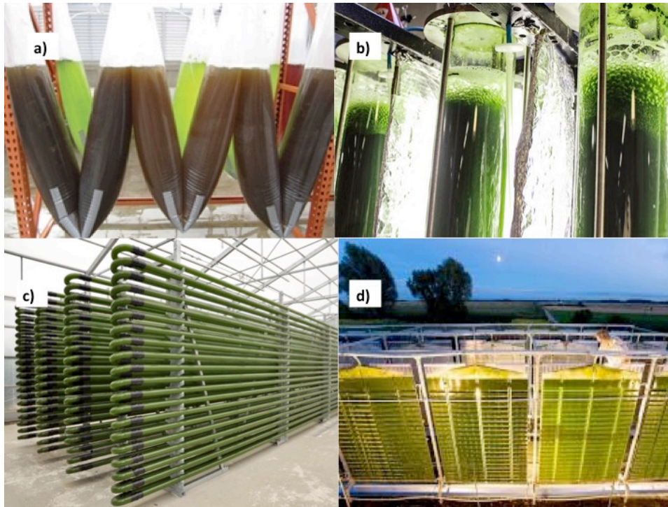
Figure 9 Photobioreactors: (a) Polyethylene bags, Le fremer Institute; (b) Vertical columns, University of Cape Town; (c) Tubular photobioreactor at the IGB Biotech; (d) Flat pannel developed by Subitech GmbH (Germany).
